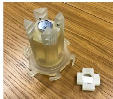
Figure 5: Prototype of target holder, containing a  $^{44}\text{Sc}$  target capsule, with a stacked degrader lying next to it.
