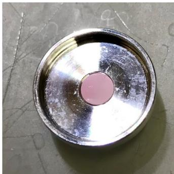
Figure 6: Pressed salt target, 6 mm in diameter, nestled in the indentation of an Al (99.5 % pure) capsule.
