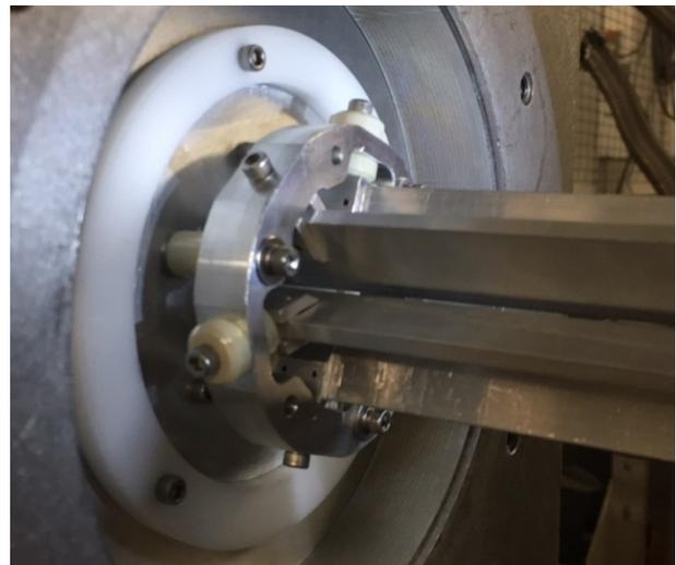
Figure 7: Vaned SPIG and pumping baffle.
