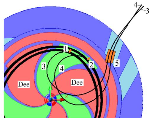
Figure 5: Extraction protons from K280 by stripping foil: 1 – the foil location for extraction of 60 MeV protons, 2 – the foil location for extraction of 70 MeV protons, 3 – trajectory of 60 MeV protons, 4 – trajectory of 70 MeV protons, 5 – bending magnet for steering proton beams with output energy in the range 60-70 MeV.
