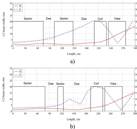
Figure 6: Extracted beam envelopes with energy of 70-MeV (a) and 60-MeV protons (b).
