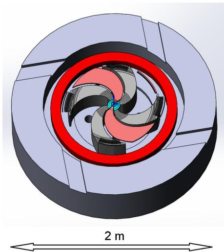
Figure 1: Cyclotron magnetic system.
