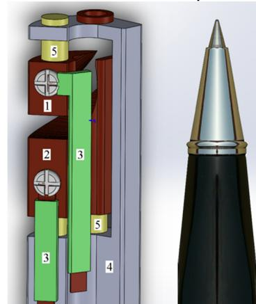
Figure 2: Structure of spiral inflector: 1 – upper electrode, 2 – lower electrode, 3 – potential connections, 4 – electrode fixation, 5 – ceramic isolators.
