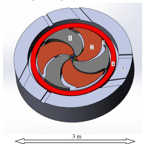
Figure 3: Cyclotron K280: 1 – sector, 2 – dee, 3 – valley shim, 4 – coil, 5 – yoke.
