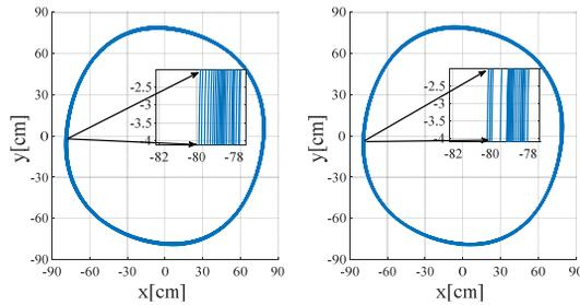
Figure 6: Left: the acceleration orbit without harmonic field. Right: the acceleration orbit When the amplitude of the harmonic field is 12 Gs and the phase is  $45^\circ$ . The turn separation increases obviously.
