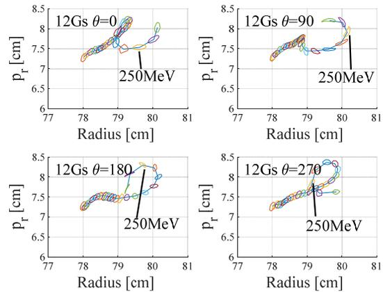
Figure 4: The phase diagrams (12 Gs  $\theta_0=0^\circ \sim 270^\circ$ ). Phase space motion with precession near the extraction region.
