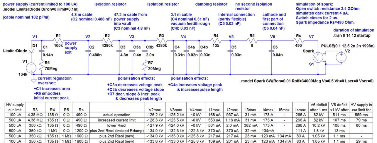
Figure 1: Present electrical circuit. Rs chosen to approximate calculated curves in Fig. 5 by V6. Its value corresponds to arc resistance at passing 75 kV. C4b, C5, C6 estimated from geometry. Simulation results are given for variants as well.
