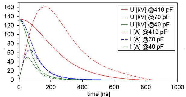
Figure 5: Voltage and current during sparkover.
