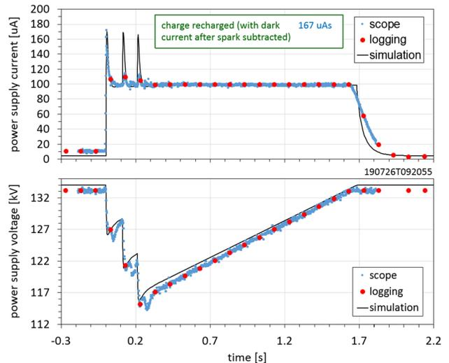
Figure 4: Triple breakdown.
