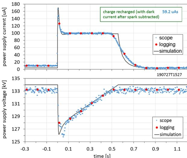
Figure 3: HV supply load curves for a “standard” spark. Current and voltage readings from HV supply analogue outputs at a scope. In addition, the data logged by the control system and the results from the LTspice simulation from Fig. 1 are depicted.
