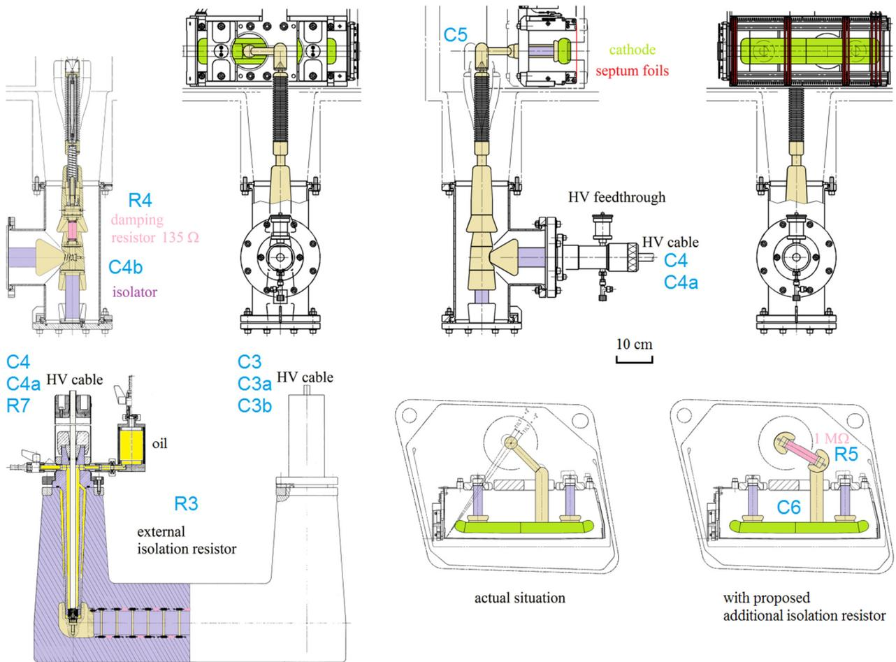
Figure 2: Mechanical setup of injection septum EIC of the Ring cyclotron. Shielded HV cables of type 2134 [9].
