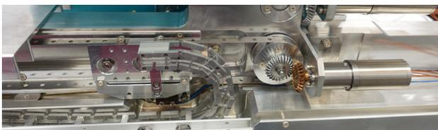
Figure 5: Test setup with motor, drive belt and an earlier version of drag chain installed.
