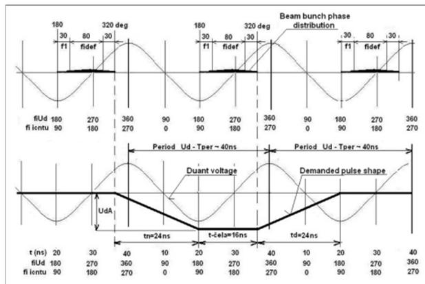
Figure 3: Time structure of the HV pulses.
