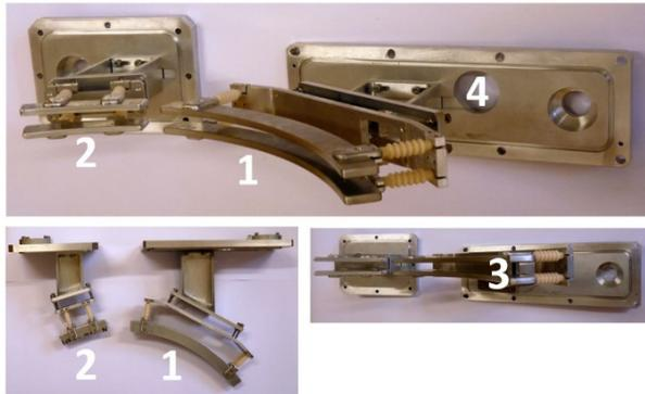
Figure 2: Two section of the deflection bunching system. 1) 1st deflector section, 2) 2nd deflector section, 3) beam entry, 4) beam exit window.
