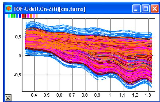
Figure 4: Vertical motion of the deflected ion during first period after HV pulse.
