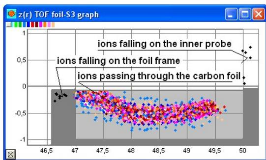
Figure 7: Ion beam distribution in the stripping foil area.
