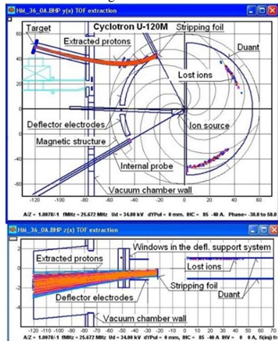
Figure 1: TOF extraction system arrangement.
