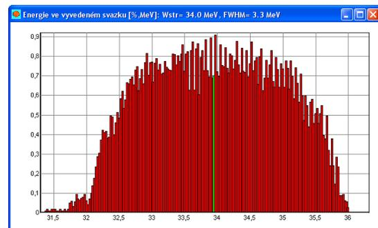
Figure 6: Extracted beam energy dispersion.
