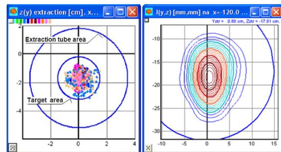
Figure 5: Extracted beam cross-section at the Be target.
