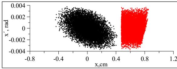
Figure 6: Horizontal plane (x,x'). Accelerated beam – left, beam at ESD entrance – right.
