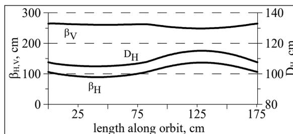
Figure 5: Horizontal  $\beta_H$ , vertical  $\beta_V$  betatron functions and horizontal dispersion function  $D_H$ .  $W = 4.8$  MeV/u.
