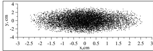
Figure 10:  $^{209}\text{Bi}^{38+}$  ion distribution in plane (x,y) at final point of extraction beam line.
