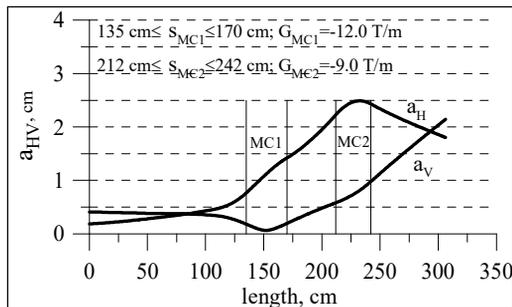
Figure 9: Horizontal ( $a_H$ ) and vertical ( $a_V$ )  $^{209}\text{Bi}^{38+}$  beam envelopes along the extraction orbit.
