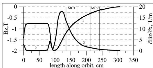
Figure 4: Cyclotron magnetic field  $B_z$  (curve 1) and its gradient (curve 2) distributions along the extraction orbit.
