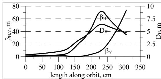
Figure 8: The betatron  $\beta_{H,V}$  and dispersion  $D_H$  functions along the extraction orbit.
