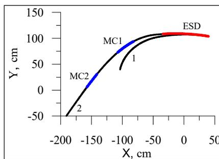
Figure 3: Closed (curve 1) and extraction (curve 2) orbits of DC140 cyclotron.
