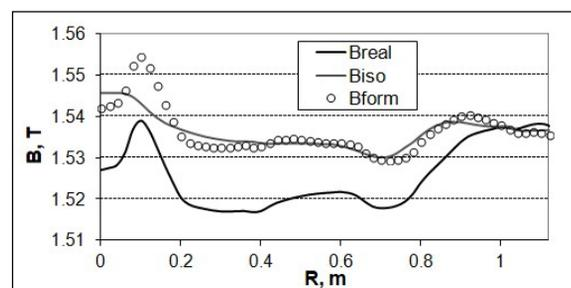
Figure 1: Magnetic fields for acceleration of  $^{209}\text{Bi}^{38+}$  ions. Breal – magnetic field formed by main coils; Biso – isochronous magnetic field; Bform – magnetic field formed by main and correcting coils.
