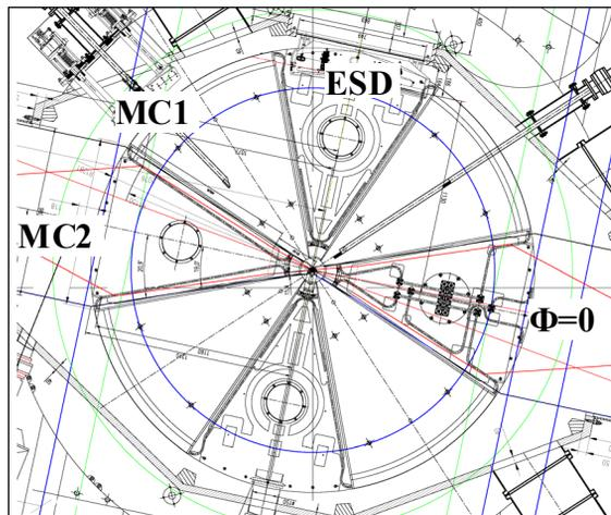
Figure 2: DC140 cyclotron working region. ESD – electrostatic deflector; MC1 – passive magnetic channel; MC2 – permanent magnet channel.
