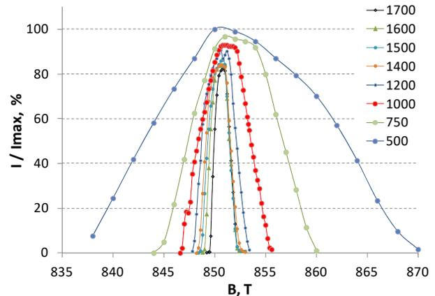
Figure 7: The dependence of relative current of  $84\text{Kr}^{14+}$  beam on magnetic field level at different radiuses.
