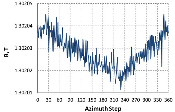
Figure 4: Signal from Hall probe at cyclotron centre.
