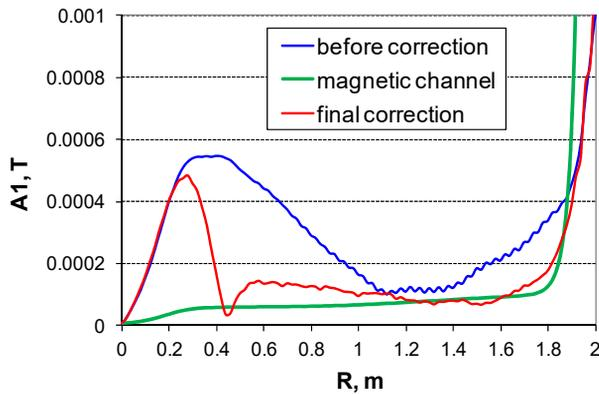
Figure 6: The amplitudes of first harmonic before and after correction and caused by magnetic channel installation.
