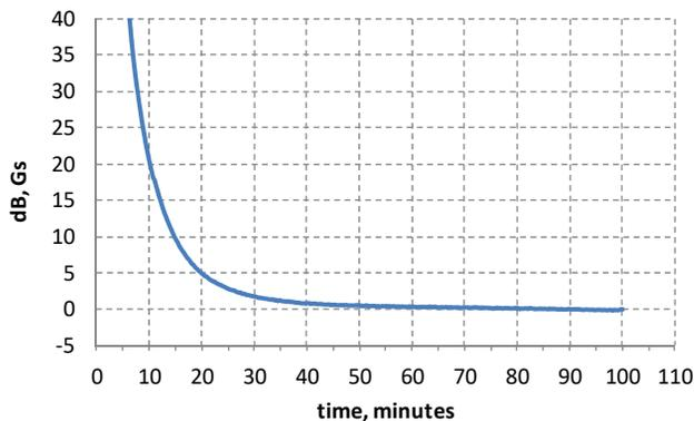
Figure 3: The time of magnetic field stabilization.
