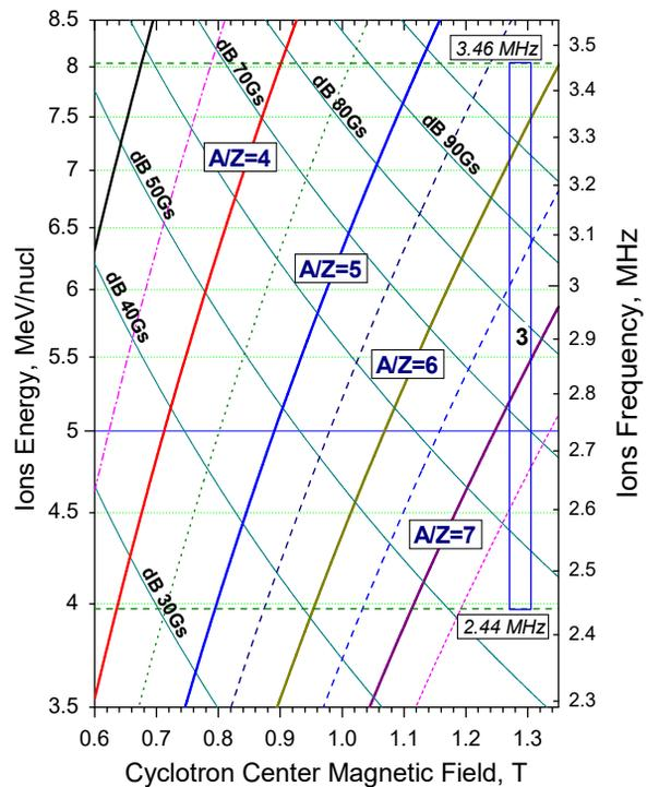
Figure 1: DC-280 Working diagram.
