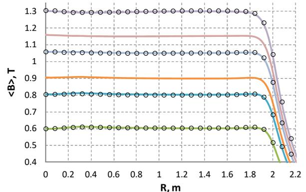
Figure 5: The calculation of the average magnetic field (circles) and the results of the measurements (line).
