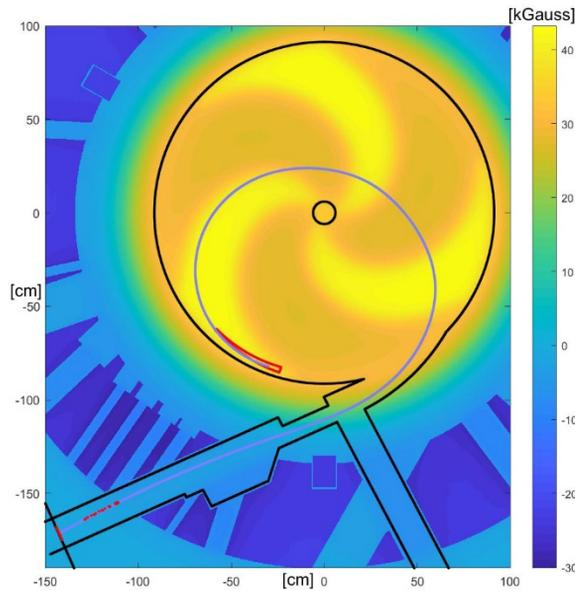
Figure 3: Fully stripped beam trajectory (light blue line) superimposed in magnetic field map (colour map), vacuum chamber (black line), stripping area (red line) and beam losing point (red dots). (mettere line nere e line rosse, togliere titolo, mm negli assi)
