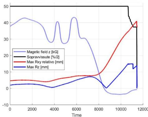
Figure 4: Beam behaviour along the fully stripped trajectory.
