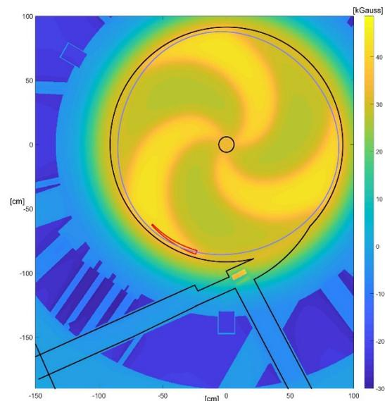
Figure 2: Magnetic field map of the cyclotron with vacuum region delimited by black line, foil region in red and stationary trajectory in blue.
