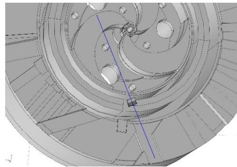
Figure 7: 3D magnetic simulation drawing of half of cyclotron joke, superconductive coil and MC1s, blue line is the reference for the magnetic field profile with which MC1s need to be optimized.
