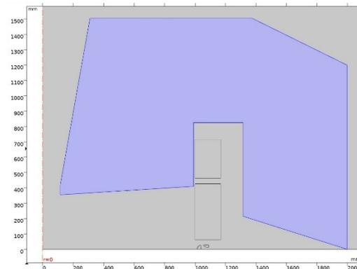
Figure 8: 2D geometry able to provide same magnetic field profile of 3D simulation, low carbon steel 1010 in light blue, the two rectangular superconductive coils, and close to the middle plane at coordinate  $r = 0$  and  $y = 1000$  the drawing of the magnetic channel.
