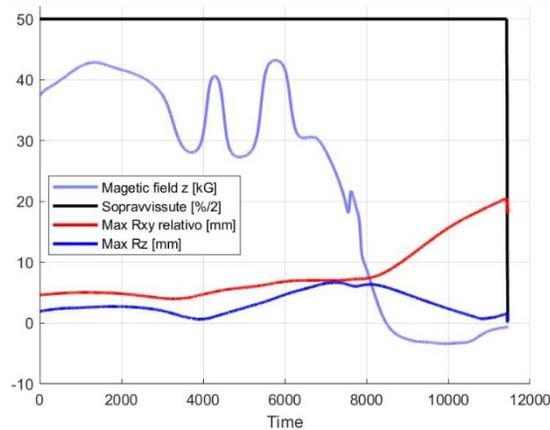
Figure 11: Beam behaviour along the fully stripped trajectory in the case of new MC1s.
