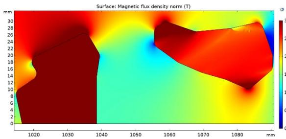
Figure 5: Slice of 3D magnetic field in correspondence of the MC1s centre.
