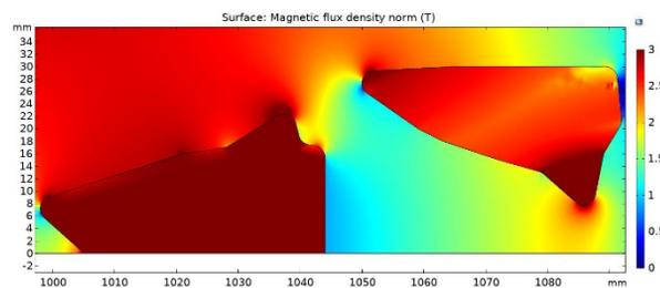
Figure 9: Slice of 3D magnetic field in correspondence of the MC1s optimized with 3D-equivalent method.
