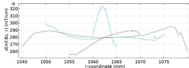
Figure 10: 3D magnetic field gradient at the centre of new MC1s.
