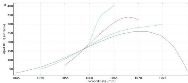
Figure 6: 3D magnetic field gradient at the centre of MC1s, see the text for the meanings of the lines.
