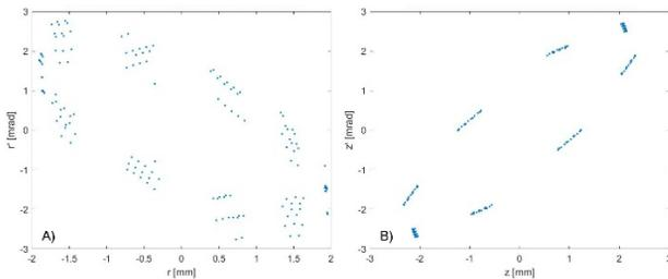
Figure 1: Auto-ellipse beam particle distributions of  $^{18}\text{O}^{6+}$  at 45.6 AMeV, A) radial phase-space diagram, B) vertical phase-space diagram.
