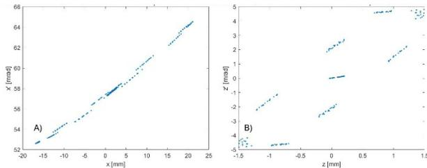
Figure 12: Beam particle distributions of extracted  $O_{18}^{6+}$  at 45.6 AMeV, A) radial phase-space diagram, B) vertical phase-space diagram.
