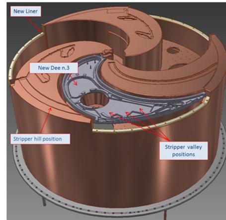
Figure 3: The stripper devices positions.
