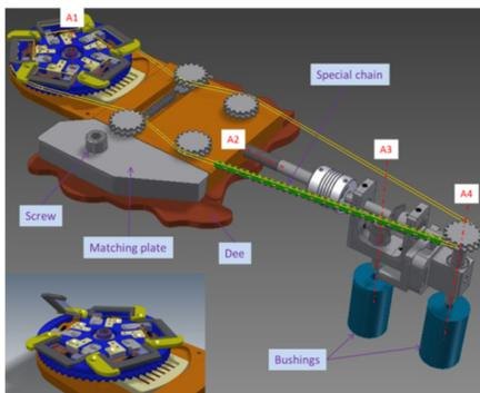
Figure 2: The valley stripper device.
