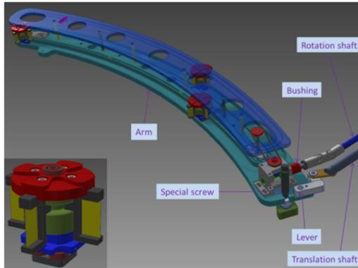
Figure 4: The hill stripper device.
