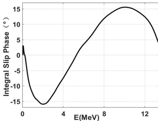
Figure 6: Integral phase slip of the final shimming.
