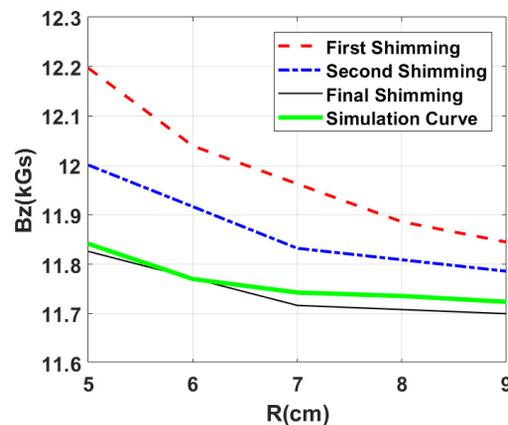
Figure 4: Average magnetic field of shimming results in the BNCT cyclotron.
