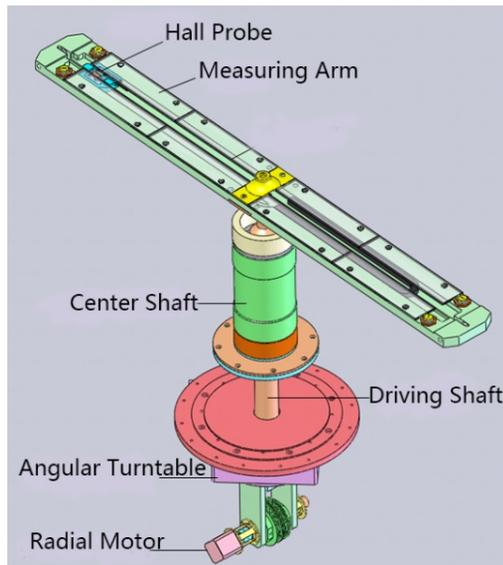
Figure 1: Mechanical structure of the measuring instrument.
