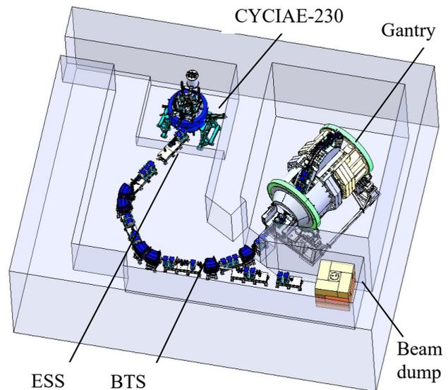
Figure 1: Layout of CYCIAE-230 and beam lines.
