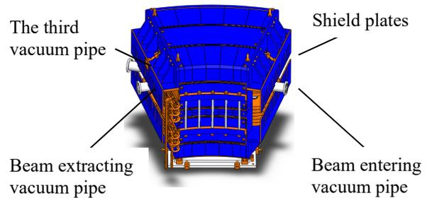
Figure 3: Model diagram of 30°-dipoles.
