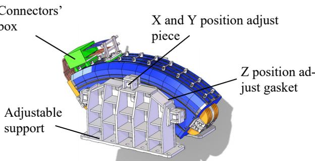
Figure 5: Model diagram of 75°-dipoles.
