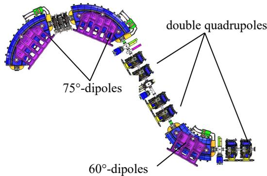
Figure 4: Layout of beam line on gantry.
