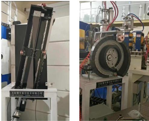
Figure 2: Photos of two types of energy degrader (left: wedge right: circle).
