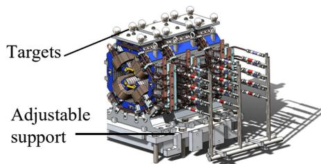
Figure 6: Model diagram of thin-thick-thin triple quadrupoles.
