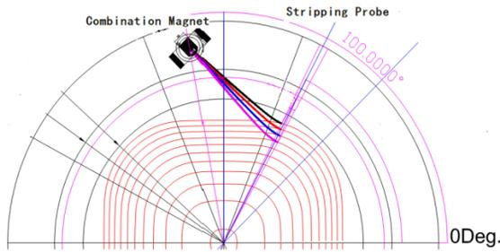
Figure 1: Stripping probe and position of combination magnet. (The red lines are equilibrium orbits).
