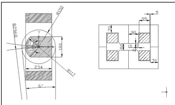
Figure 6: The structure of the combination magnet.
