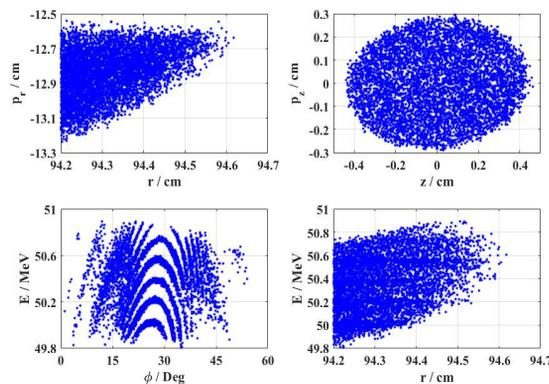
Figure 4: The extracted beam phase space distribution for 50 MeV on the stripping foil.
