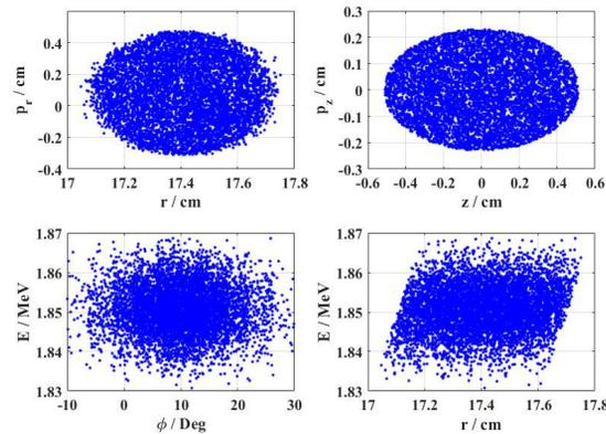
Figure 3: Initial phase space distribution with the normalized emittance of  $4.0 \pi \cdot \text{mm} \cdot \text{mrad}$  and phase width of  $\pm 20^\circ$ .
