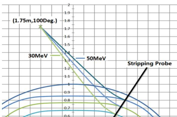
Figure 2: The extracted trajectories with the combination magnet fields for different energies.
