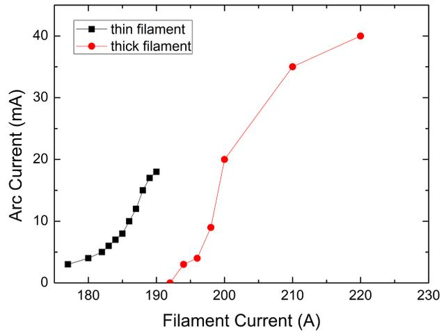
Figure 4: Arc current versus filament current.
