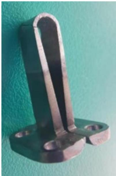
Figure 6: Fracture of thick filament at high current.
