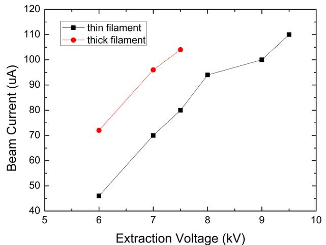
Figure 5: Results of beam extraction experiments of thin filament: beam current versus dc extraction voltage.
