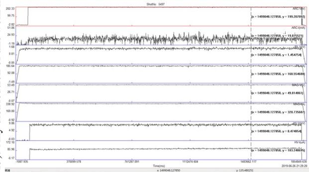
Figure 7: Waveform collected of the stable ion source discharge.
