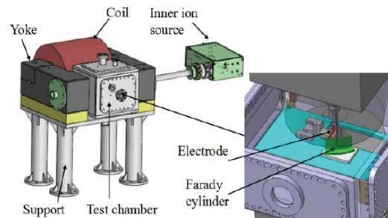
Figure 1: The components of the ion source test bench.
