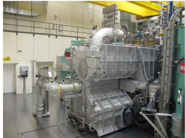
Figure 3: The new 50 MHz Resonator 2 installed in the Injector 2 Cyclotron.
