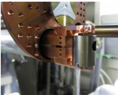
Figure 3: High-temperature oven (HTO) used in the 28-GHz superconducting ECR ion source (SC-ECRIS).
