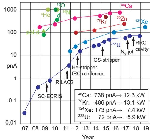
Figure 8: Evolution of the beam intensity at the exit of the SRC since the start of operation of RIBF in 2007. The maximum intensity achieved so far is presented for  $^{48}\text{Ca}$ ,  $^{78}\text{Kr}$ ,  $^{124}\text{Xe}$ , and  $^{238}\text{U}$  beams, along with the corresponding beam power. The main R&D items for increasing the uranium beam are also indicated.
