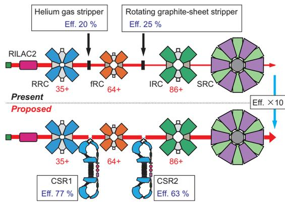
Figure 10: Present (upper panel) and proposed (lower panel) accelerator chains for the uranium beam at RIBF. The present stripping efficiency is 5%. Replacing the two charge strippers with charge stripper rings (CSR1 and CSR2) is expected to increase the total stripping efficiency to about 50%.
