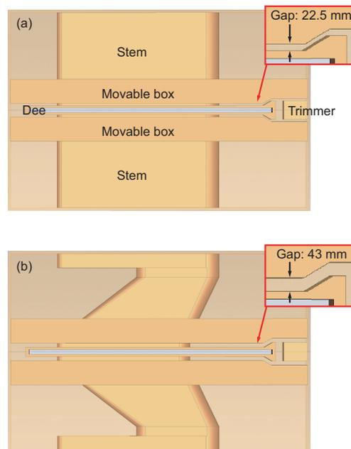
Figure 5: Calculation models for the original cavity (upper panel) and the modified cavity (lower panel). The gap length required for a resonant frequency of 18.25 MHz is shown in each panel.
