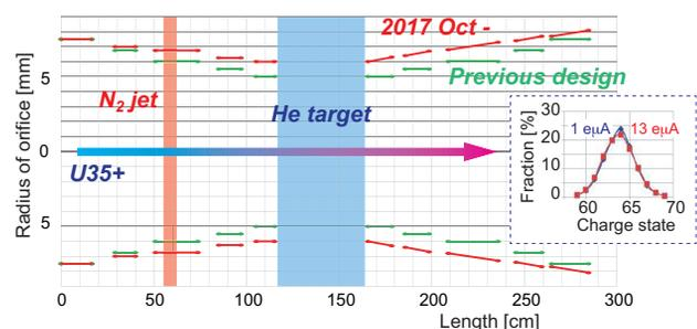
Figure 4: Orifice diameters in the helium gas stripper. The green lines represent the orifice diameters in the original structure. The  $N_2$  gas-jet has expanded the orifice diameters to those represented by the red lines.
