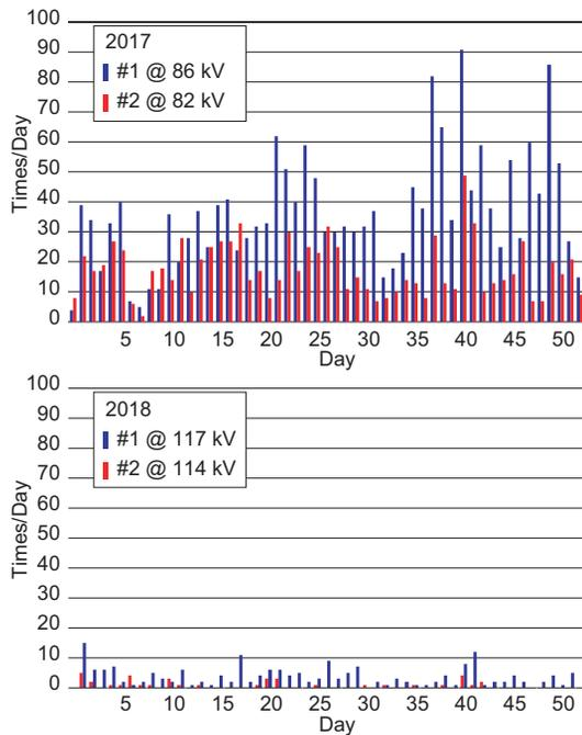
Figure 7: Comparison of frequency of voltage breakdown during the uranium beam time in 2017 (upper panel) and that in 2018 (lower panel). After the modification in 2018, the frequency of the breakdown decreased significantly despite the increased acceleration voltage.
