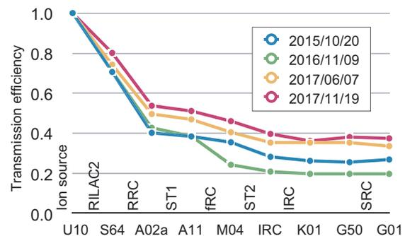
Figure 9: Transmission efficiency during uranium beam acceleration. The horizontal axis corresponds to the position of the Faraday cups in the accelerator chain. Note that the stripping efficiencies in the charge strippers are not included in the transmission efficiency.
