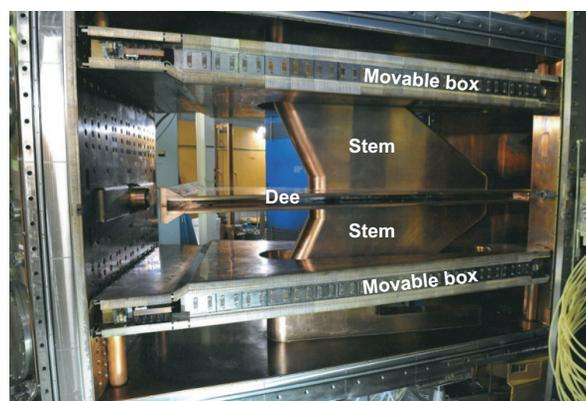
Figure 6: Internal view of the modified RRC cavity.
