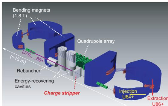
Figure 11: Schematic drawing of the charge stripper ring, optimized for the second stripping stage at the RIBF.
