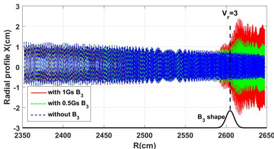
Figure 7: The radial beam profile during acceleration with and without third harmonic field near the  $\nu_r=3$  resonance.
