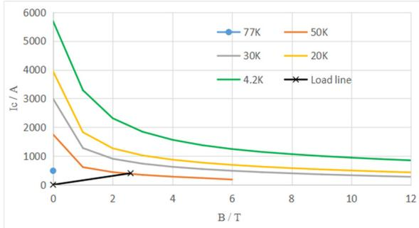
Figure 11: The load line of the HTS superconducting coil for the defocusing magnet.
