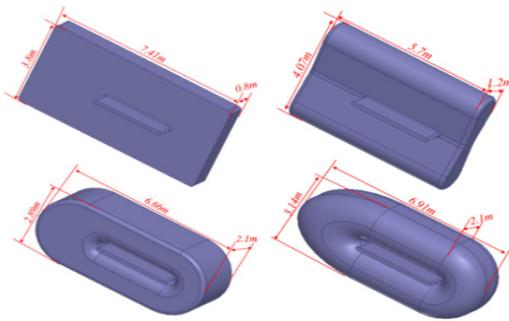
Figure 13: Four geometries of the waveguide-type cavity.
