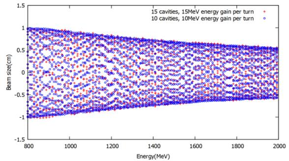
Figure 8: The radial beam profile with 10 and 15 cavities for acceleration.
