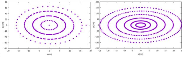
Figure 5: The radial (left) and vertical (right) phase space at 800 MeV.
