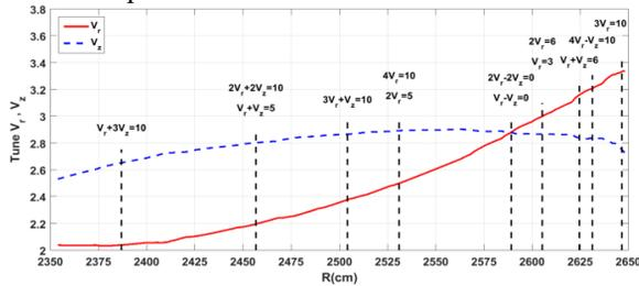
Figure 6: The tune values varying with radius and the main resonances crossed in the machine.
