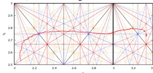
Figure 3: Tune diagram.
