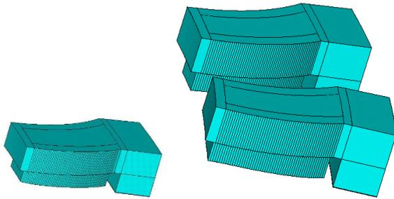
Figure 10: The 3D model of the defocusing magnet and the two focusing magnets.
