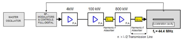
Figure 12: One typical module of the high-power RF system for the 2GeV FFAG.
