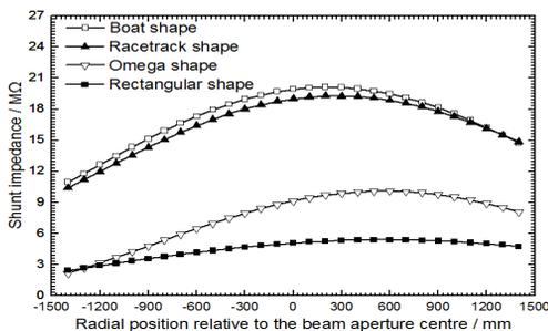
Figure 14: Relationship between the shunt impedance and the radial position relative to the aperture centre.
