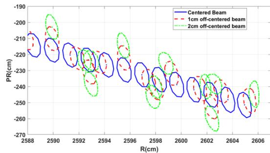
Figure 9: The radial phase space during accelerator with centered, 1 cm off-centered and 2 cm off-centered beam.
