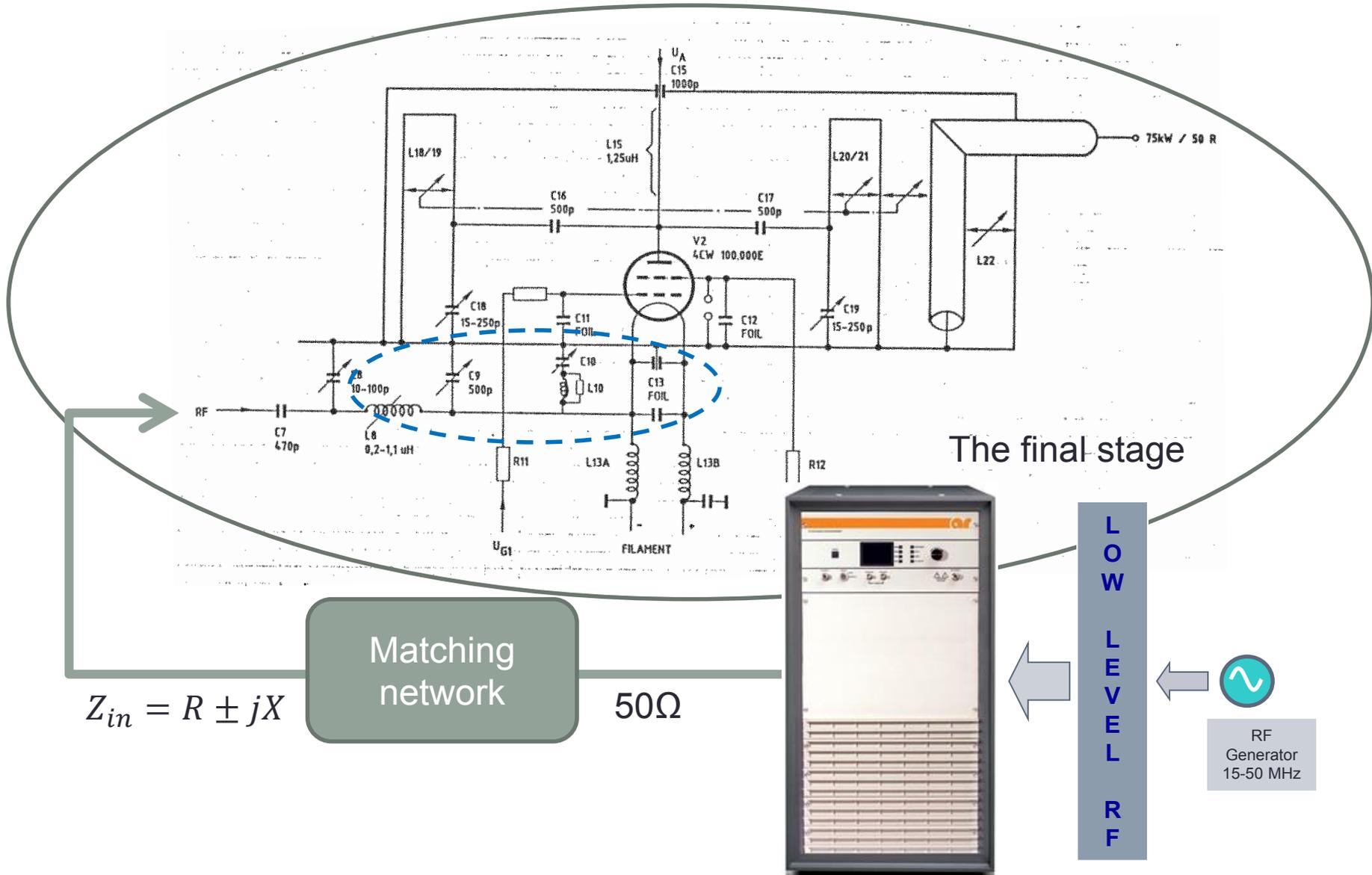
We need a matching network as impedance transformer from  $Z_0$  to cathode impedance  $Z_c$
