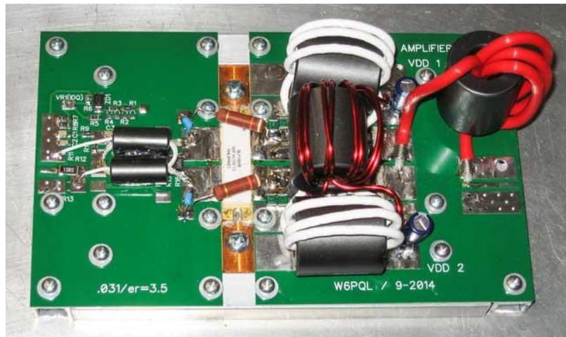
Output Power  $\geq 1kW$
