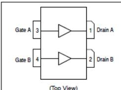
Note: The backside of the package is the source terminal for the transistors.
