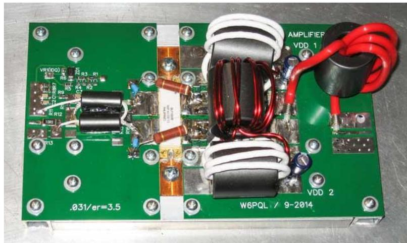
Output Power  $\geq 1kW$
