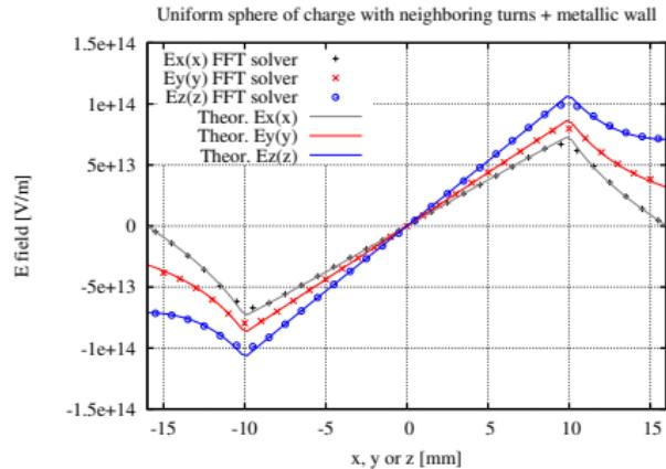
Dots are from our Poisson solver ( $32 \times 32 \times 32$  grid,  $10^6$  particles); solid lines are from theory. Note the three different boundary conditions in  $x$ ,  $y$ , and  $z$ : periodic, open, and metallic.
