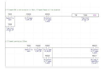
Figure 5. Ladder diagram of vacuum tube ON sequences
