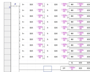
Figure 4. Ladder diagram of Vacuum pressure calibration
