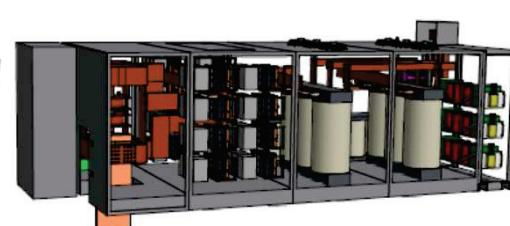
The TRIUMF application requires short term stability for the current in the order of two part per million (ppm) of nominal (20 kA), after the first five minutes following a current change. Repeatability must be of the same order and current ripple must be within ±2 ppm of 20 kA for the range from 17 kA to 20 kA.
