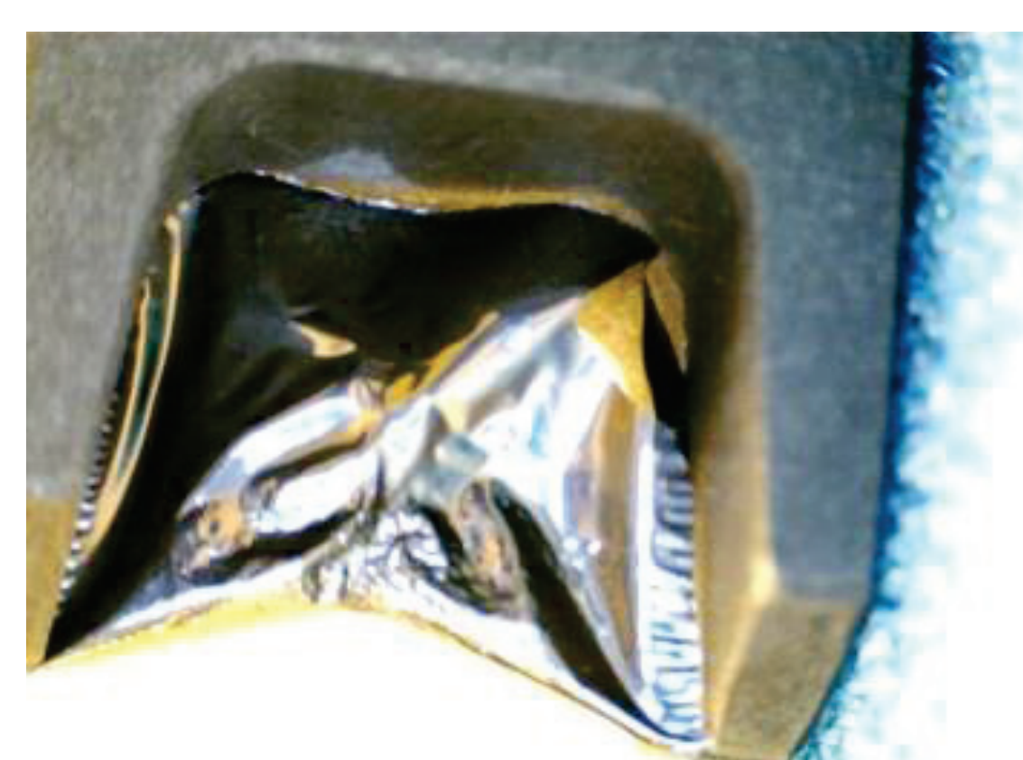
The picture of broken graphene foils after 16,000 \mu\text{A}\cdot\text{Hour}
