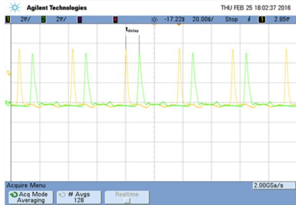
Figure 6: TOF measurement from FCT1 and FCT 2.
