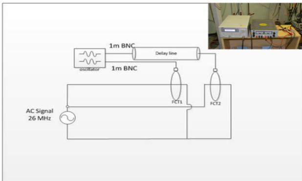
Figure 5: Arrangement of capacitive pickup to perform calibration of the experiment setup.
