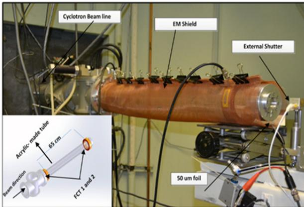
Figure 4: Experimental setup for energy measurement. The two FCT can be seen under the copper mesh. The distance between them is 65 cm. the purpose of the EM shield is to reduce electromagnetic noise.
