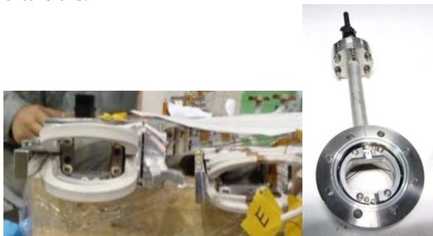
Figure 3: Examples of baffle slit extension: left figure shows magnetic channel slit extended from 15 mm X 15 mm to 33 mm X 30 mm and right figure shows slit of B in figure 4 which extended from 30 mm X 24 mm to 36 mm X 30 mm.
