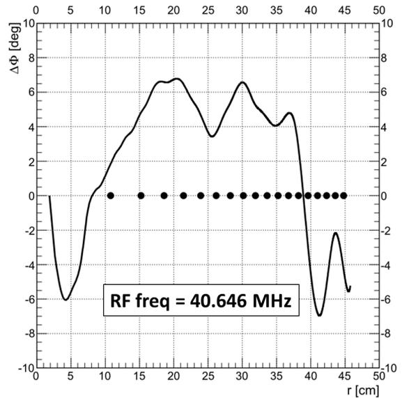
Figure 8: The integrated phase slip as a function of the average equilibrium orbit radius in the prototype Cyclone<sup>®</sup> KIUBE
