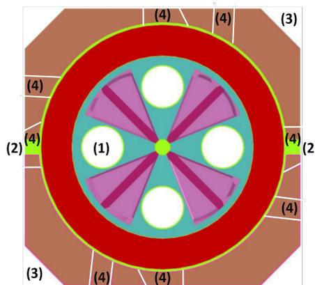
Figure 2: A top view on the Cyclone<sup>®</sup> KIUBE. 1/ the four pumping holes in the valleys, 2/ the coil electrical and cooling ports, 3/ the yoke lifting system and 4/ the extraction ports.
