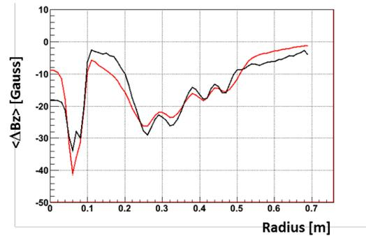
Figure 5: Comparison of a calculated and measured magnetic effect after milling of the pole insert.
