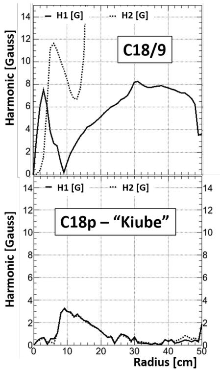
Figure 6: The 1st and 2nd harmonics in the measured magnetic map: (top) in the Cyclone<sup>®</sup> 18/9 and (bottom) in the Cyclone<sup>®</sup> KIUBE. The large harmonic 2 in the Cyclone<sup>®</sup> 18/9 is due to the presence of movable iron inserts in the valleys.
