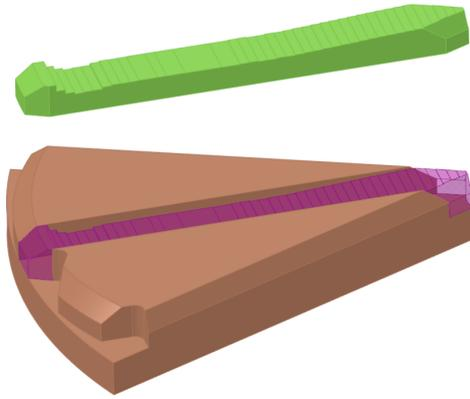
Figure 3: A view on the Cyclone<sup>®</sup> KIUBE pole. A groove is present in the middle of the pole to accommodate the pole insert. The pole insert is shown as well, where the milling profile on the face closest to the median plane is visible. The azimuthal length of the pole is 45 degrees and gradient corrector cuts on the pole outer border are present to facilitate the extraction from the cyclotron (see [2]).
