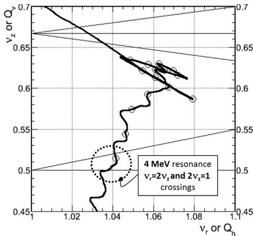
Figure 7: Tune diagram of the Cyclone<sup>®</sup> KIUBE.
