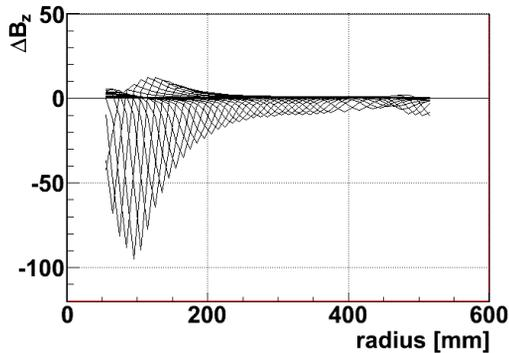
Figure 4: The effect on the average field of iron milling on the pole insert. These curves correspond to 24 identical cuts of 10 mm radial width and 5 mm depth on different radial positions.
