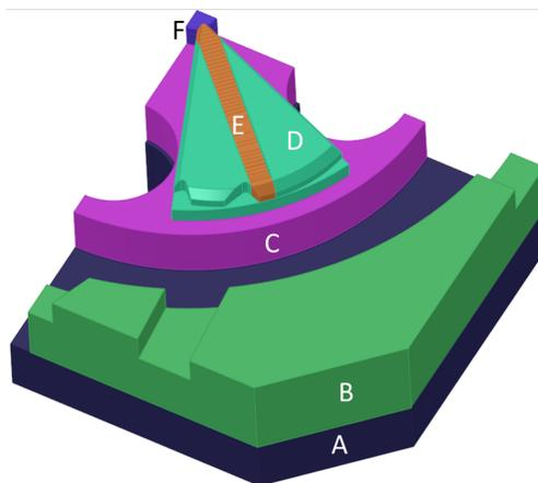
Figure 1: The magnetic circuit, including (A) the return yoke, (B) lateral return yoke, (C) sector, (D) the pole, (E) the pole insert and (F) the central plug.
