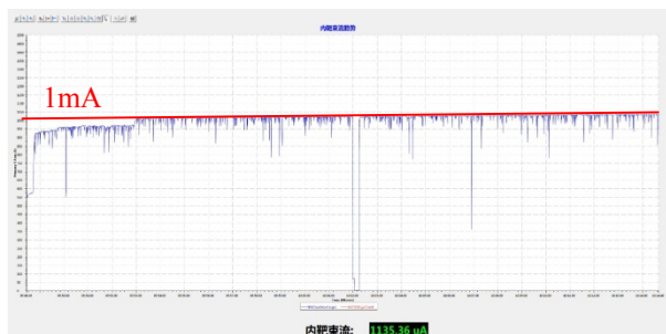
Figure 8: The beam current history measured by the internal target at 1 MeV.
