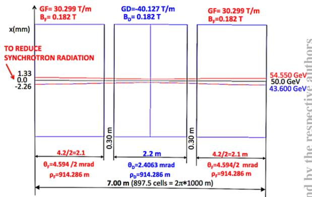
Figure 4: Orbit offsets in the higher energy range LHeC NS-FFAG ERL proposal with magnet properties: gradients and bending angles.
