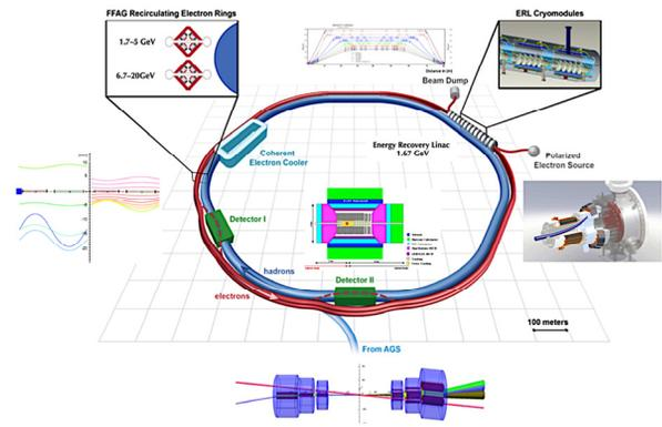
Figure 5: *eRHIC* layout with major components.
