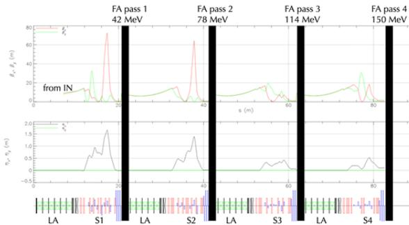
Figure 11: Simulation of the 8 passes through the CBETA linac, spreader and combiner, NS-FFAG with the energy recovery.
