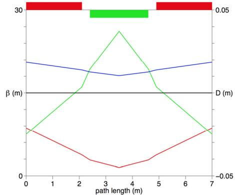
Figure 3: Betatron functions for the central energy of the higher NS-FFAG ERL design, with the combined function magnets.
