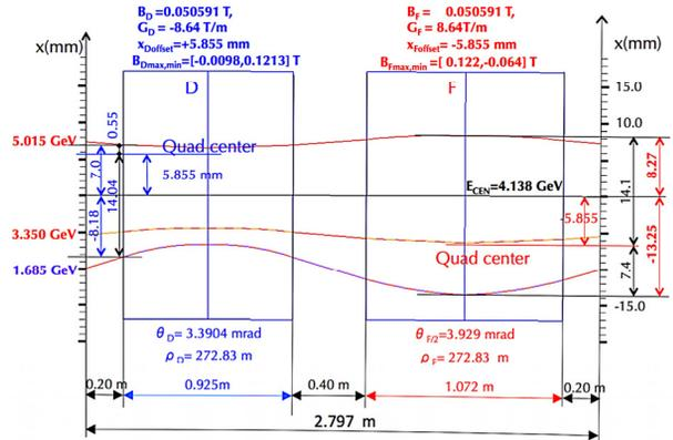
Figure 6: Orbit offsets in the basic cell for the NS-FFAG design for the larger energy range 6.68-20 GeV.
