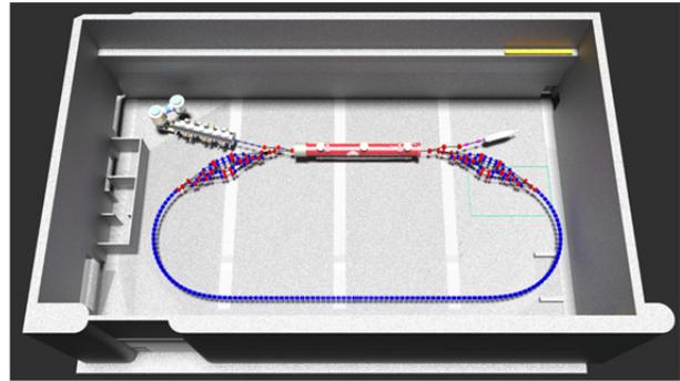
Figure 9: Layout of the eRHIC prototype at Cornell University (CBETA). The upper left corner shows the injector, followed by the Linac (red colour), following with a dump. On both sides of the linac there are a combiner (on the left side) and spreader on the right side. The NS-FFAG arc and straight section is shown by blue color.
