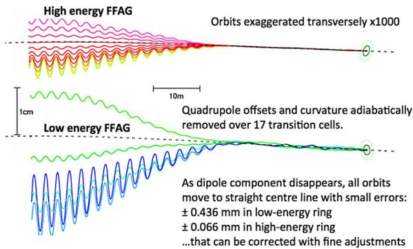
Figure 7: New property of the NS-FFAG lattice: Adiabatic removal of the quadrupole offsets and matching to the straight section.
