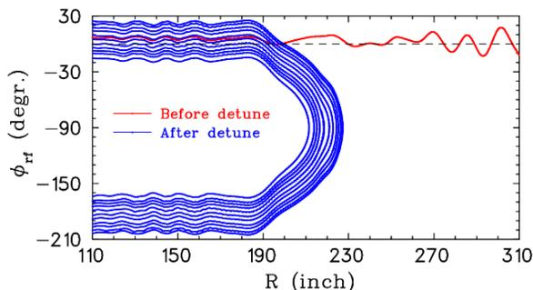
Figure 5: Phase space diagram of beam deceleration.
