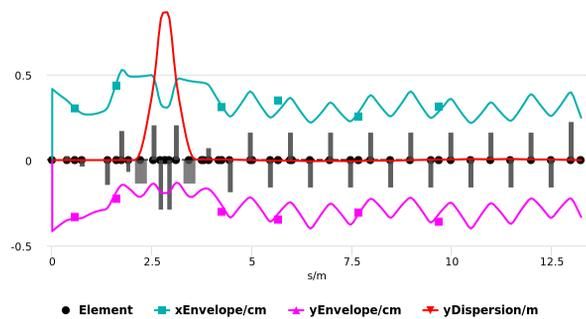
Figure 3: Beam envelope trough 1/3 of injection line; squares represent beam size at profile monitors.
