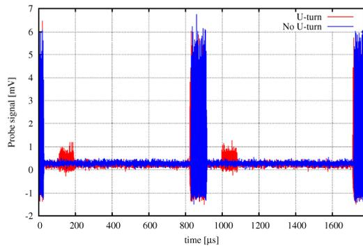
Figure 6: BL2C4 extracted beam: blue – no deceleration, red – with deceleration.
