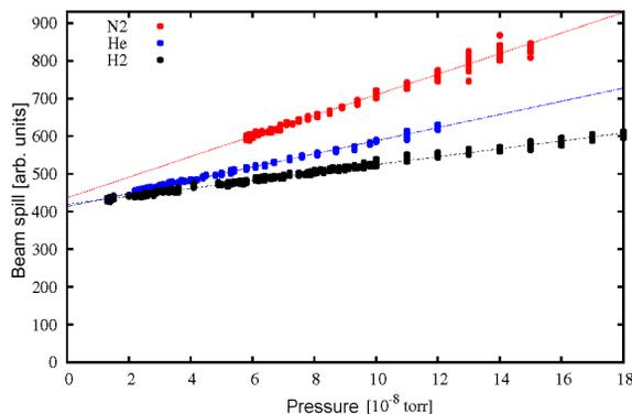
Figure 7: Beam spill vs partial pressure of some gases
