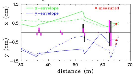
Figure 8: BL2A beam envelope: dashed lines – old tune; solid lines – new tune.
