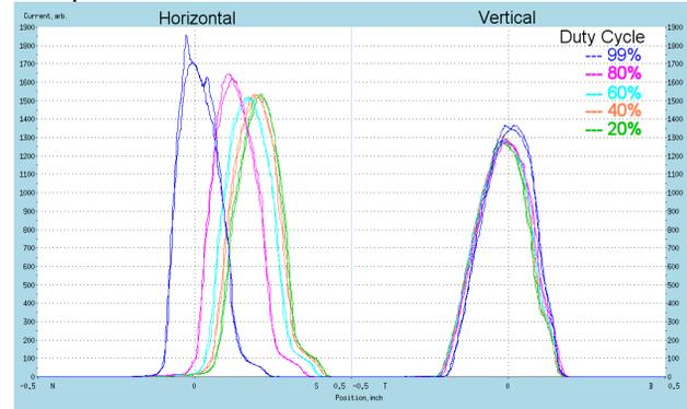
Figure 2: Beam horizontal steering vs duty cycle.
