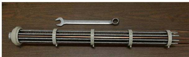
Figure 5: The 1 m RF ion conveyor with a 1-1/4" wrench for scale.
