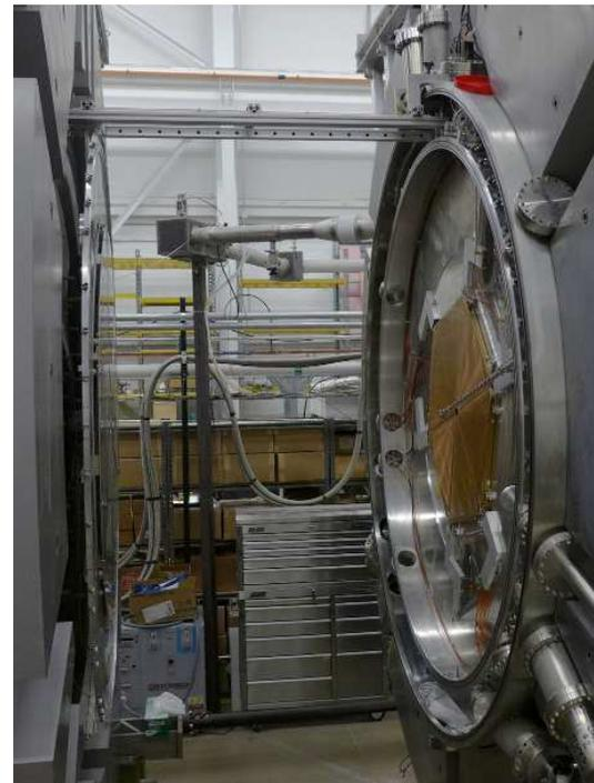
Figure 4: Closeup showing the stopping chamber with the RF ion carpets installed inside the opened cyclotron stopper.
