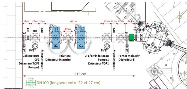
Figure 6: Elements composing the beamline. Q1/Q2: quadrupole 1/2. SV1: steerer.
