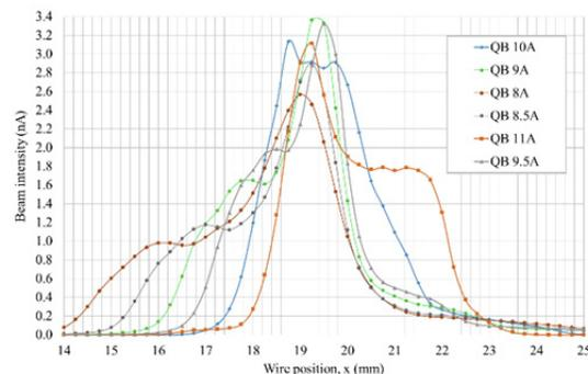
Figure 3: Beam profile at 18 MeV.
