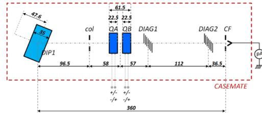
Figure 2: The quad scan setup (distances are in cm).
