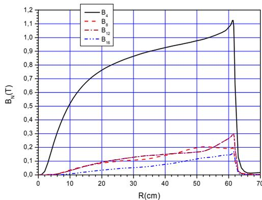
Figure 5: Multiple Fourier harmonics of cyclotron magnetic field.
