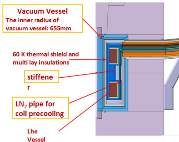
Figure 9: Preliminary design sketch of the cryostat.
