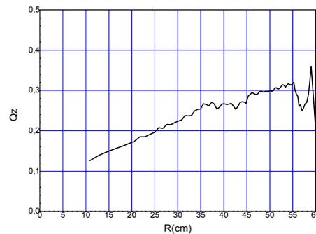
Figure 7: Vertical betatron frequency for the isochronous cyclotron magnetic field.
