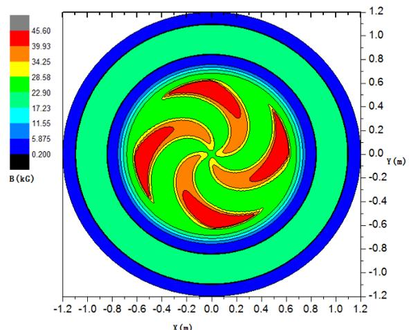
Figure 2: Contour plot of median plane magnetic field.
