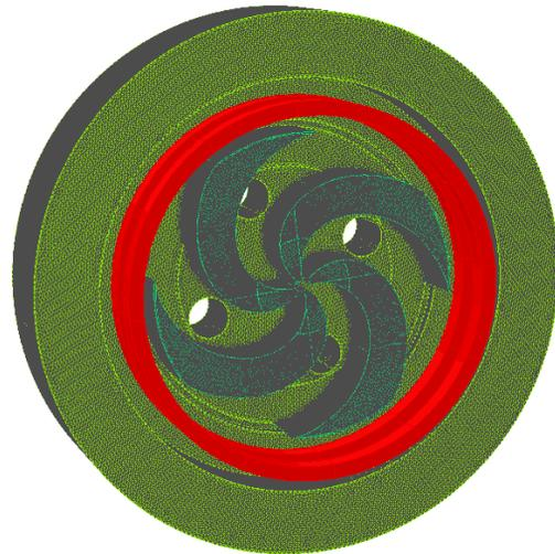
Figure 1: Layout of the TOSCA model for SC200 cyclotron.
