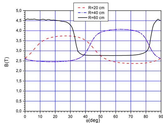
Figure 8: SC200 magnetic field for R=20, 40, 60 cm.
