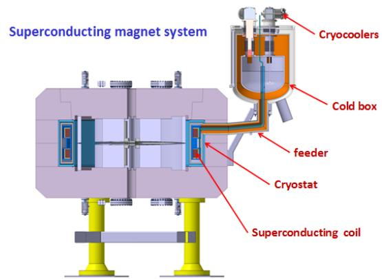
Figure 10: SC200 cyclotron magnet preliminary design.
