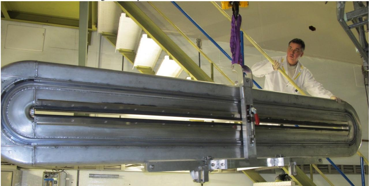
Figure 4: Transport of expandable sealing with shim for installation into the Ring cyclotron.
