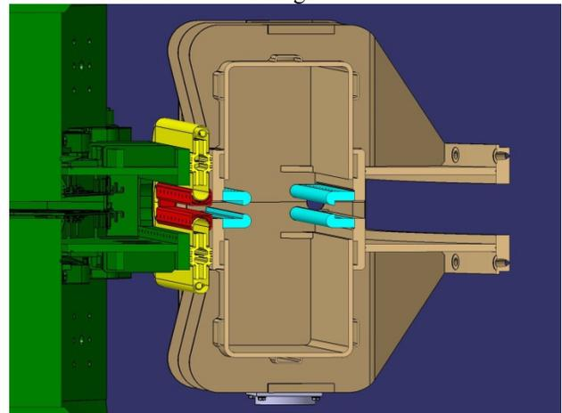
Figure 2: Cross section of flattop cavity (beige) with electrodes (cyan), expandable vacuum sealing (yellow) with shim (red) and vacuum chamber of sector magnet 6 (green).
