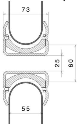
Figure 3: Cross section of expandable sealing with shim. Dimensions of vertical gap and length in mm.
