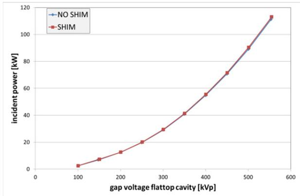
Figure 5: Incident power versus gap voltage of flattop cavity.
