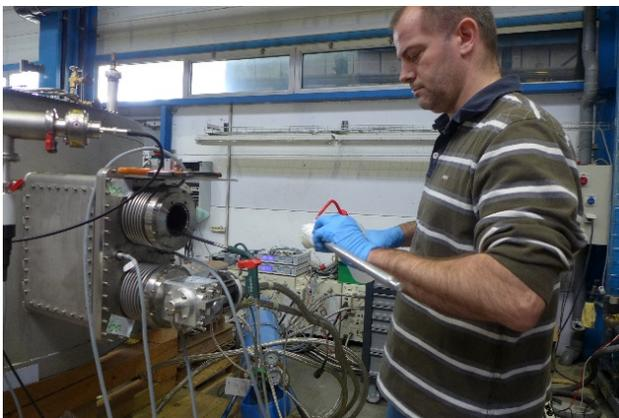
Figure 3: Cryohead maintenance with the cold swap method.
