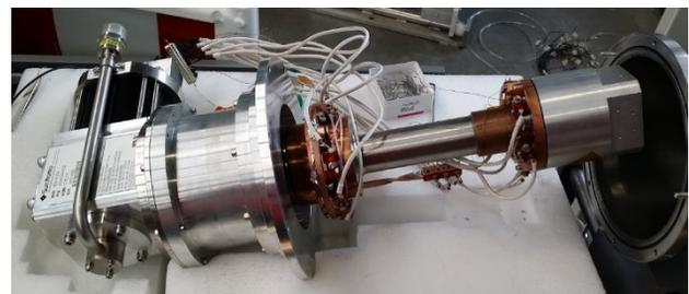
Figure 2: 1<sup>st</sup> and 2<sup>nd</sup> stage heating system.
