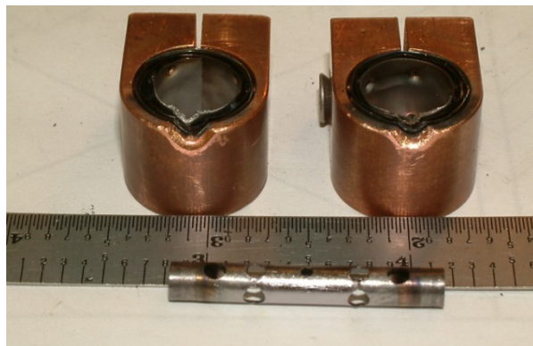
Figure 4: The copper clamps and the detached, tantalum crucible for the high-temperature oven.
