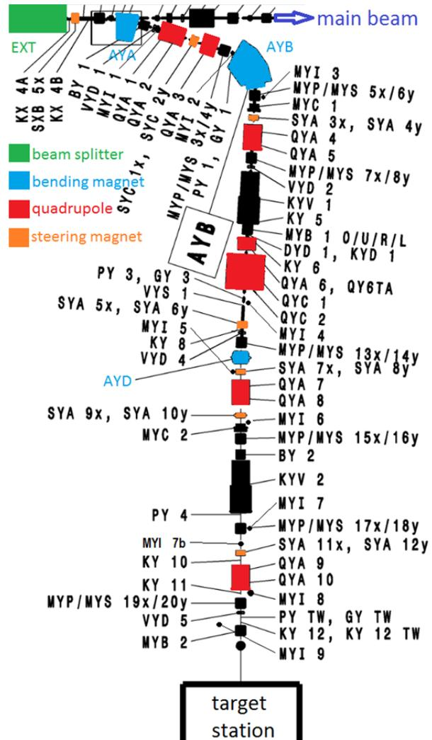
Figure 1: Isotope production beam line.
