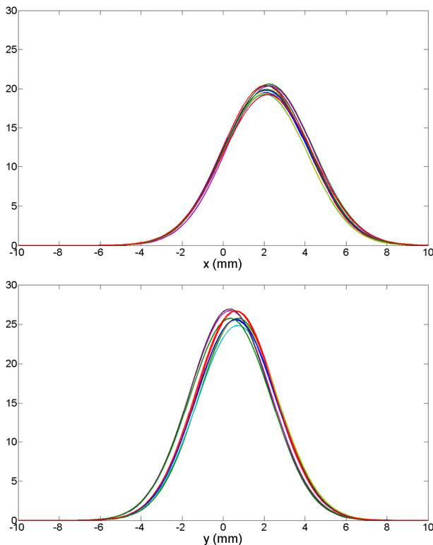
Figure 3: Ten beam profiles measured in one session. Top: horizontal; Bottom: vertical.
