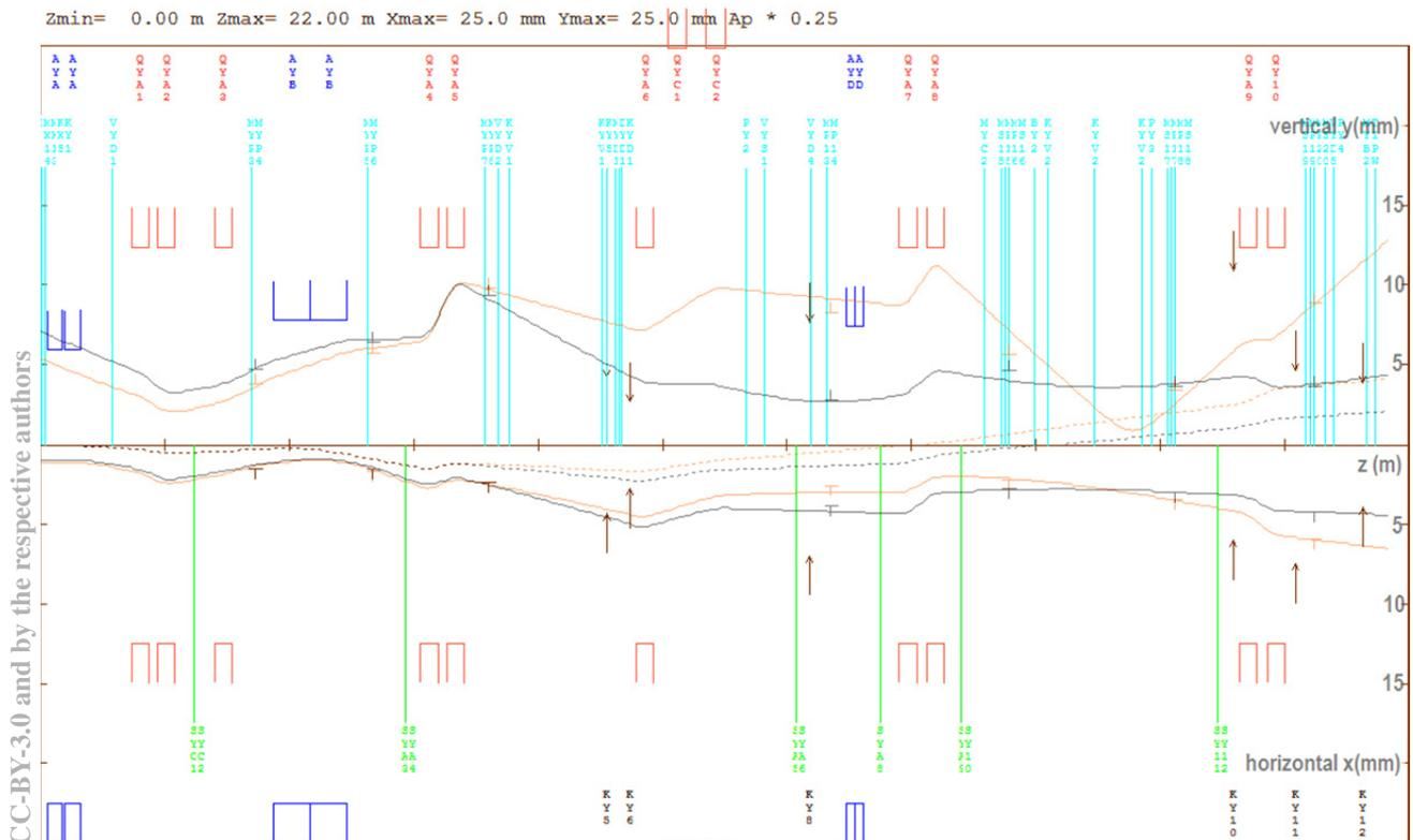
Figure 2: Beam envelopes for  $^{44}\text{Sc}$  and  $^{64}\text{Cu}$  productions in black and orange.
