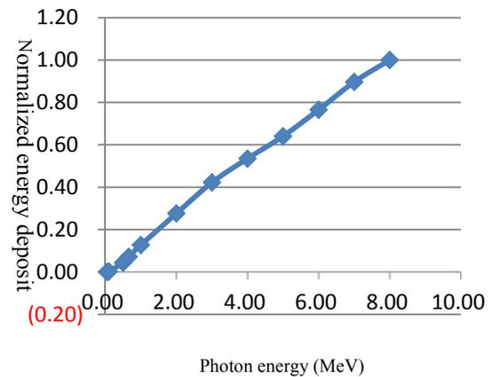
Figure 5: Energy response curve of air ionization chamber.
