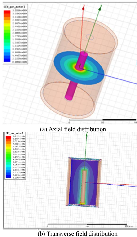
Figure 2: Electrostatic field distribution of the chamber.
