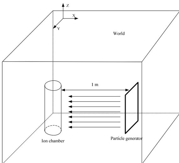
Figure 4: The Geant4 simulation model.
