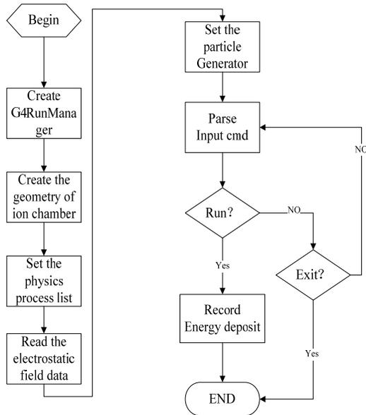
Figure 3: Flowchart of Geant4 simulation program.
