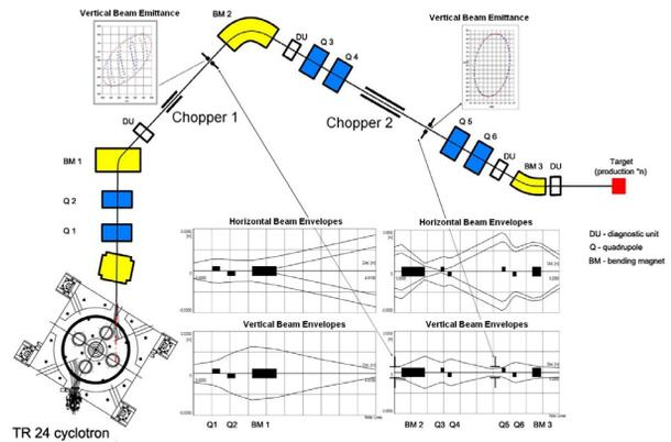
Figure 4: TR-24 external beam shopping system layout.
