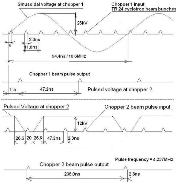
Figure 8: Timing of the deflector voltages on sinusoidal resp. pulsed chopper.
