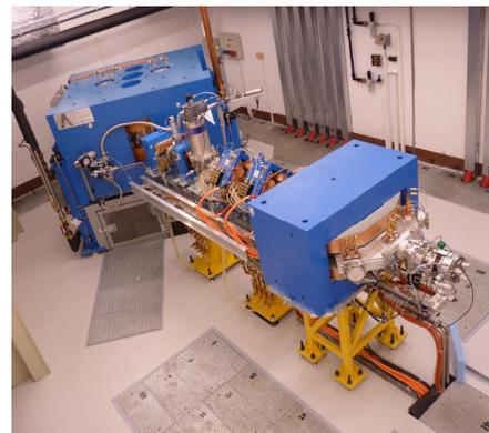
Figure 2: Cyclotron TR 24 with the beam line.
