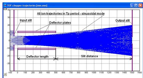
Figure 6: Sinusoidal deflection system arrangement.
