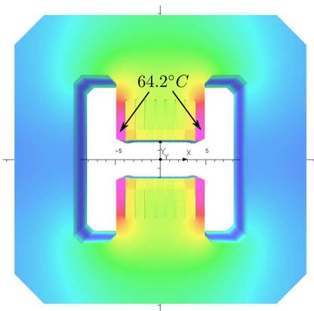
Figure 6: The temperature distribution of the optimized SMX magnet.
