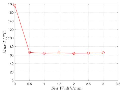
Figure 5: Maximum temperature of the SMX magnet vs. slit width.
