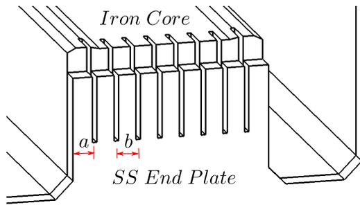
Figure 4: The distribution of slits in the SMX magnet.
