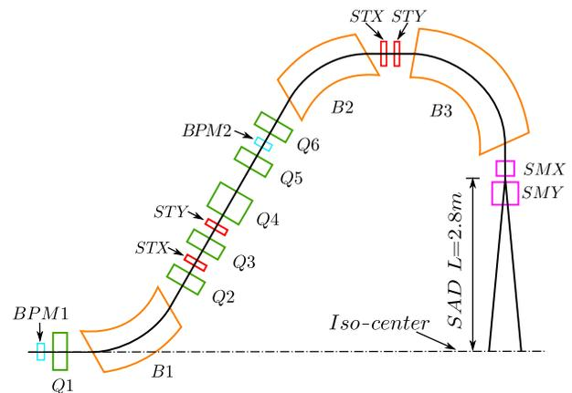
Figure 1: The layout of the rotating gantry and the illustration of the SAD length.
