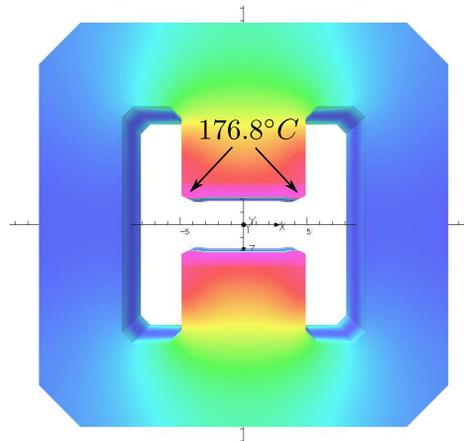
Figure 2: The temperature distribution of the unoptimized SMX magnet. The maximum value concentrates on the pole edge.
