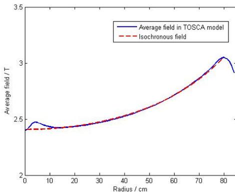
Figure 3: The average magnetic field in TOSCA model after sectors shaping.
