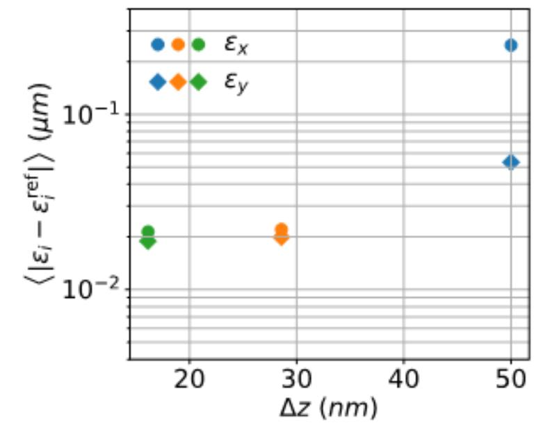
Grid resolution  $\Delta x = \Delta y = 10 \mu\text{m}$  and  $\Delta z = 28.6 \text{ nm}$  was chosen
