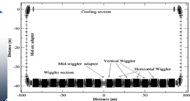
FIG. 2. Layout of the ring cooler.
