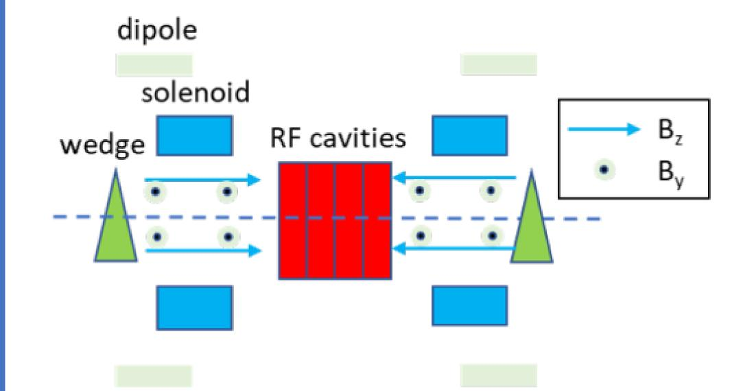
The whole cooling channel consists of 5 stages and each stage includes repeated cells. The cell length will gradually reduce for stronger focusing at the wedge absorber in order to achieve smaller emittance. Fringe field of dipole magnets is considered as well and for now a simple quadratic function is used to describe the fringe. The absorber material in all stages is liquid hydrogen and 100  $\mu m$  Be safety window is used.
