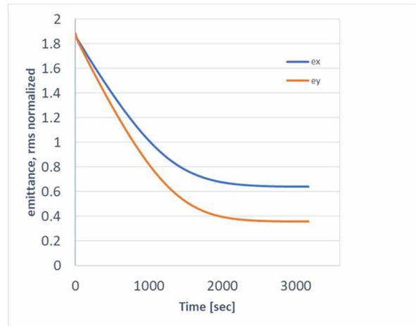
Figure 2: Cooling of protons at  $\gamma=25.4$ , with decoupled transverse motion (simulations with IBS, using single harmonic RF, and cooling only). Horizontal emittance (top curve, blue) and vertical emittance (bottom curve, orange).
