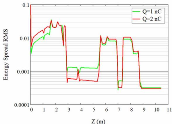
Figure 5: Simulated energy spread for electron bunch charges of 1 and 2 nC at the end of 13 MeV linac.
