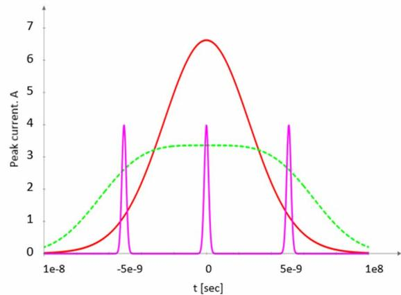
Figure 3: Three electron bunches (magenta) spaced by 5.1 ns placed on a single proton bunch (red: single RF harmonic; green: double RF harmonic).
