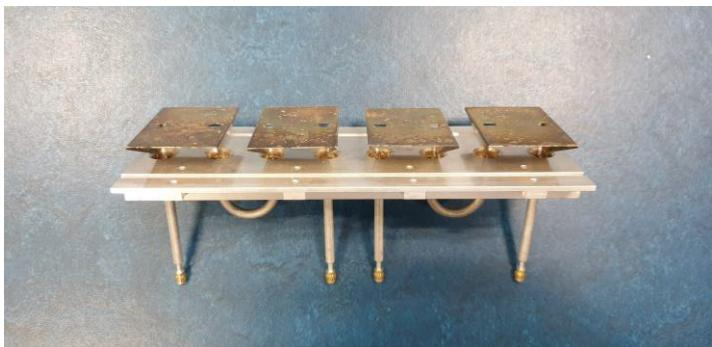
$\lambda/4$  “super-electrodes” as used in pick-up and kicker loads inside vacuum tank
