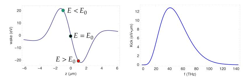
The kick generated by one proton in the kicker section. The longitudinal scale of the wake is  $z\sim 3\mu$ m, corresponding to the frequency bandwidth  $\Delta f\sim c/\pi z \approx 40$  THz. In the *optimal* settings the cooling rate is estimated as
