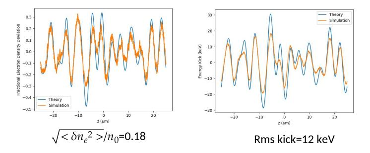
This is one of the limitations of the cooling rate. We can achieve cooling time ~2 hours with  $\sqrt{\langle \delta n_e^2 \rangle}/n_0 \sim 0.2$ .
