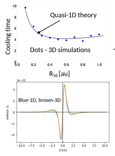
3D effects have been studied analytically<sup>\*</sup> in the case when there is no amplification. In this case, the results agree well with the quasi-1D model. No unexpected surprises found in 3D.
