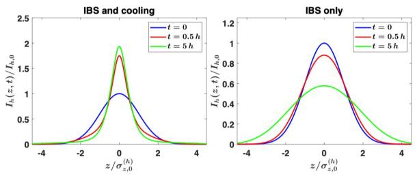
The hadron longitudinal distribution becomes narrower when the energy spread decreases due to cooling. Without cooling the hadron bunch length increases.
