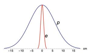
The electron bunch length is shorter than the hadron one. Hadrons with large synchrotron amplitudes spend a fraction of time inside the electron beam.
