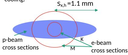
Gaussian charge distribution with different  $S_x$  and  $S_y$  corresponding to the nominal x and y proton beam emittance in EIC.
