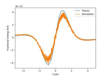
Wake for the case of one amplifier for 275 GeV protons, both from the linear theory and the average of 10 runs of the simulation. Good agreement is observed.
