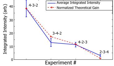
Signal intensity increases when the chicane strength is optimized. Good agreement with theory.
