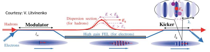
Coherent electron cooling is a variant of the stochastic cooling with the operational frequency range raised from ~GHz to tens of THz. (Derbenev, AIP Conf. Proc. **253**, 103 (1992); Litvinenko, Derbenev. PRL, **102**, 114801 (2009)).
