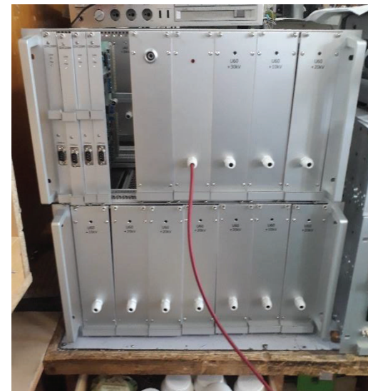
Gun-collector control electronics
