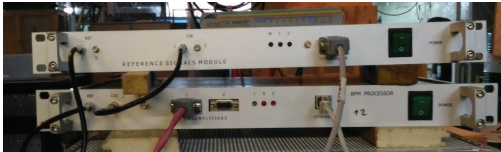
Test of BPM electronics on “Gun-Collector” test bench
