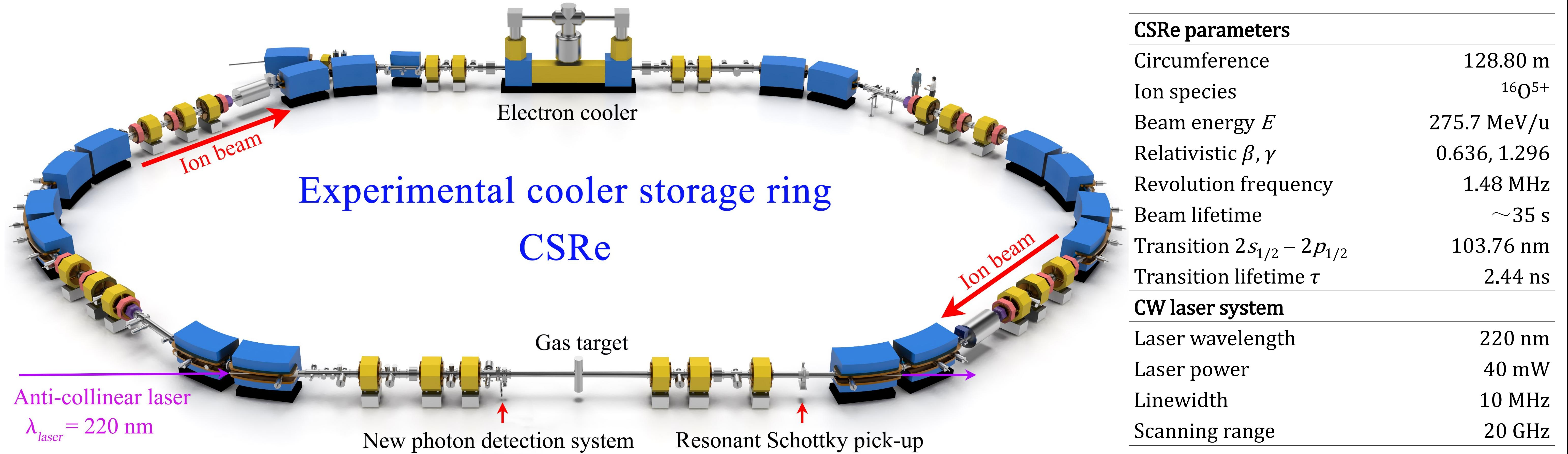
Fig.1. Schematic view of the cooler storage ring CSRe and the main parameter settings for laser cooling experiment of  $^{16}\text{O}^{5+}$  ion beams.
