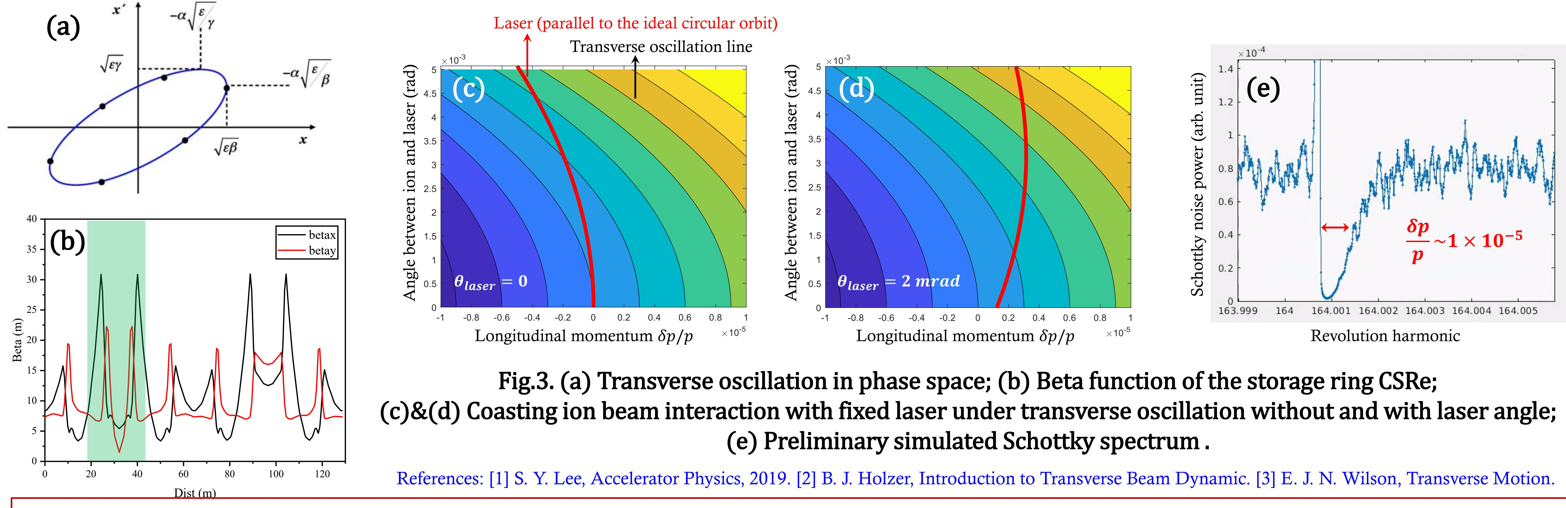
Fig.3. (a) Transverse oscillation in phase space; (b) Beta function of the storage ring CSRe; (c)&(d) Coasting ion beam interaction with fixed laser under transverse oscillation without and with laser angle; (e) Preliminary simulated Schottky spectrum .
