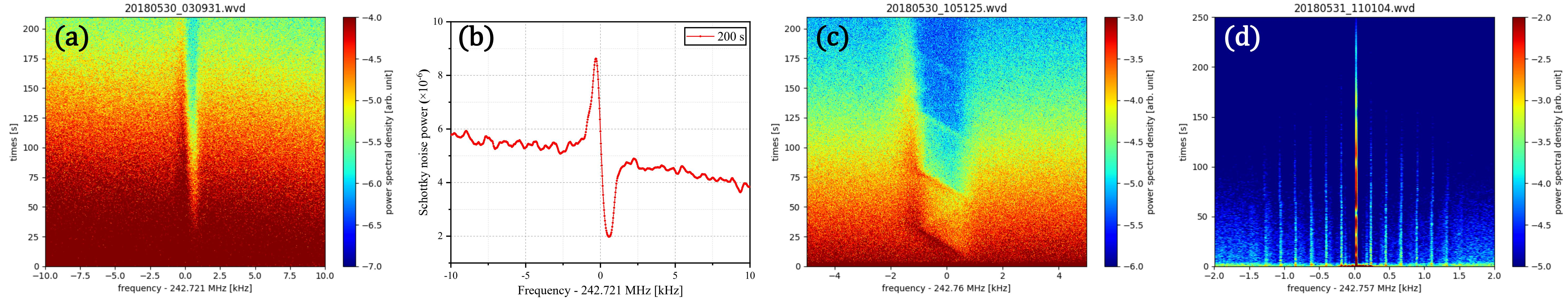
Fig.2. Experimental results: (a) coasting ion beam interaction with fixed laser; (b) 200s of (a); (c) coasting ion beam interaction with scanned laser; (d) laser cooling of bunched ion beams.
