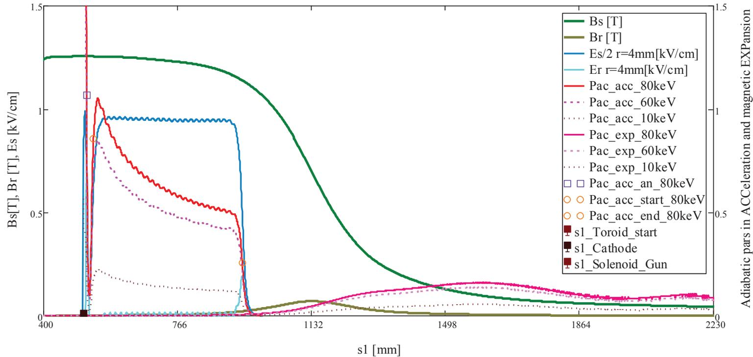
Electrons are **accelerated** with the **adiabatic parameters 1.04/0.85/0.21** in longitudinal, and **expanded** with the **parameters 0.16/0.14/0.05** in transverse at three electron energy of 80keV/60keV/10keV respectively. They met the adiabatic conditions.
