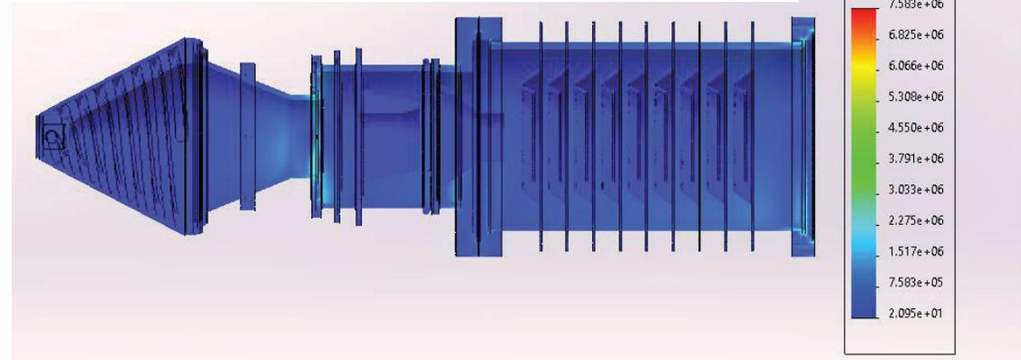
Max. deformation: 0.026mm (<1.0mm required)
