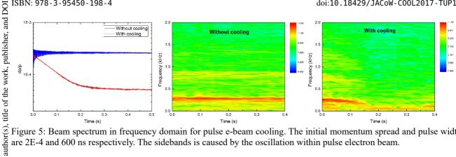
Figure 5: Beam spectrum in frequency domain for pulse e-beam cooling. The initial momentum spread and pulse width are 2E-4 and 600 ns respectively. The sidebands is caused by the oscillation within pulse electron beam.
