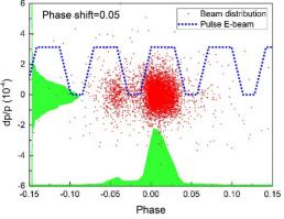
Figure 8: Beam distribution after cooling with the pulsed e-beam which have a phase shift (0.05) in longitudinal.
