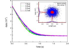
Figure 6: Cooling process with long pulse width of e-beam and the particle distribution before and after cooling.
