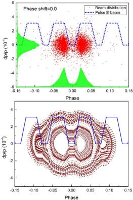
Figure 7: Beam distribution after cooled by short pulse ebeam with pulse width 20 ns and single particle tracking in phase space.
