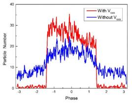
Figure 2: Final beam distribution after cooling with  $V_{kick}$  and without  $V_{kick}$ .
