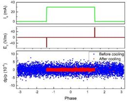
Figure 1: The distribution electron beam current and its electric potential at the edge, and distribution of particles in phase space when pulse e-beam is applied.
